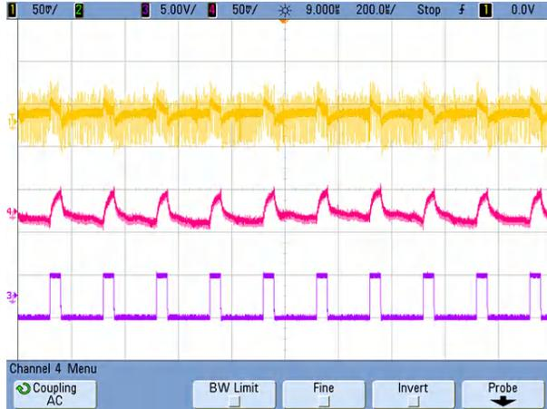
Figure 3-7. Load Transient Response of Positive and Negative Output Rail With Symmetrical Loads (25 mA)
