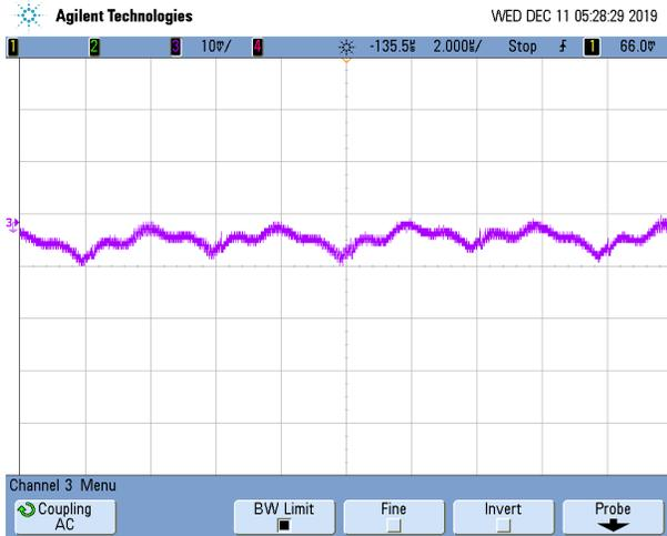
**Figure 3-3. Output Ripple of Negative Rail Before Power Filter**
