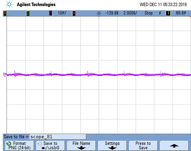
**Figure 3-4. Output Ripple of Negative Rail After Power Filter**
