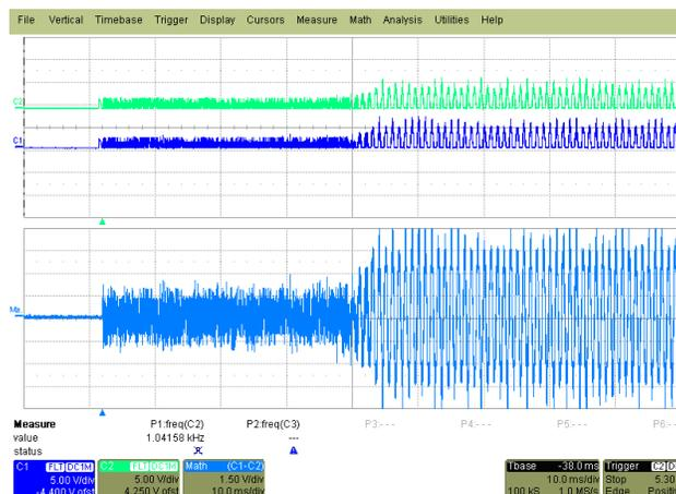
Figure 23. Volume Ramp Rate Control Enabled
