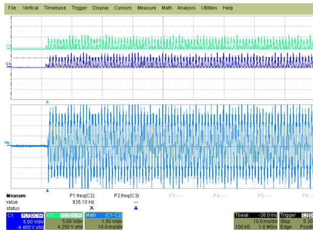
Figure 22. Volume Ramp Rate Control Disabled
