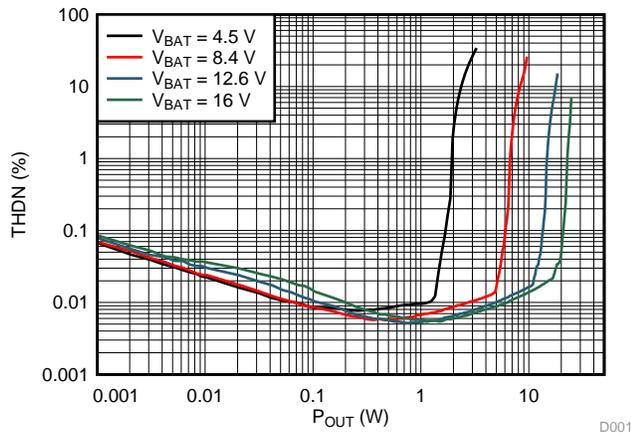
Figure 1. THD+N Performance, R<sub>L</sub> = 4 Ω, F<sub>s</sub> = 1 kHz
