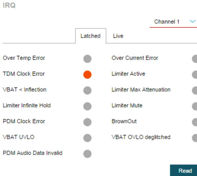
**Figure 28. Configurable Interrupts**
