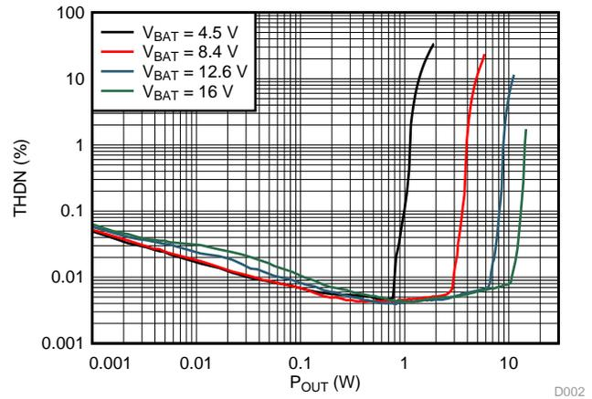
Figure 2. THD+N Performance, R<sub>L</sub> = 8 Ω, F<sub>s</sub> = 1 kHz
