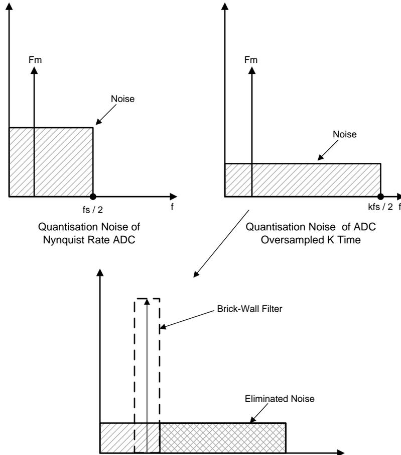
**Figure 2. Digital Filtering to Reduce the Noise After Oversampling**
