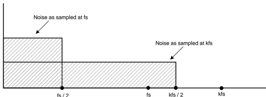
**Figure 1. Frequency Spectrum of ADC Oversampled K Times**
