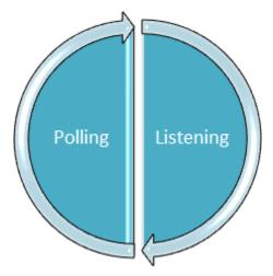
Figure 15. NFC Initiator and Target Switching Mechanism
