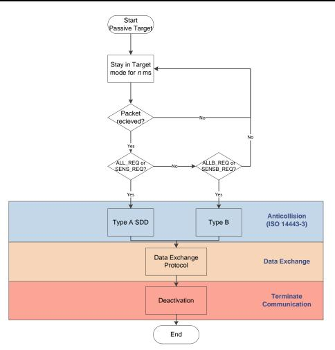
Figure 2. Card Emulation Flow Diagram
