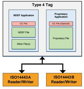
Figure 8. Type 4 Tag Structure
