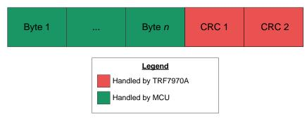
Figure 5. Frame Format for Card Emulation Type B Commands During Anticollision
