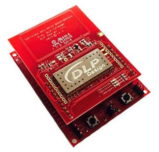
Figure 10. MSP430F5529 LaunchPad Development Kit and DLP-7970ABP BoosterPack Plug-in Module
