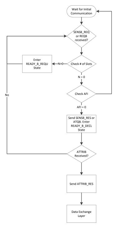
Figure 6. Card Emulation Type B Anticollision
