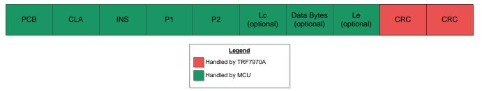
Figure 7. Frame Format for ISO 7816-4 Data Exchange Commands
