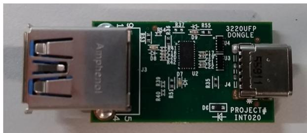
**Figure 2. HD3SS3220 UFP Dongle**
