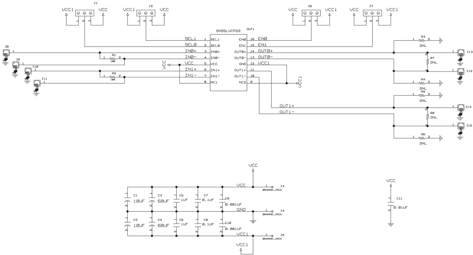
**Figure 10. SN55LVCP22EVM-CVAL Schematic**
