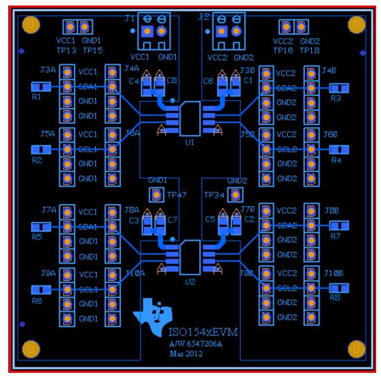
Figure 4-1. ISO154xEVM Top-layer Routing
