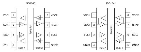
Figure 1-1. ISO1540 and ISO1541 Pinout
