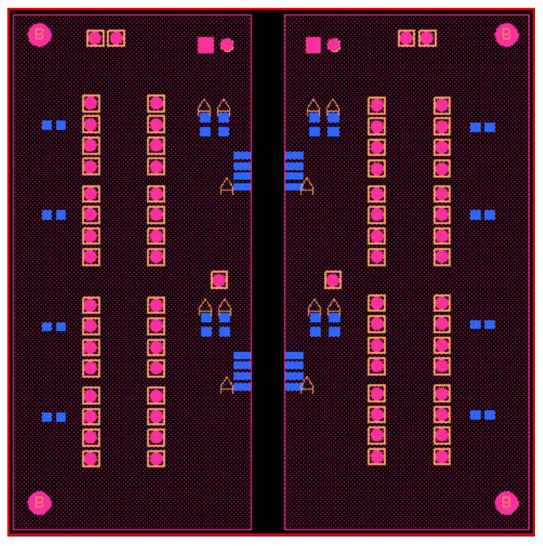
Figure 4-2. ISO154xEVM Bottom-layer Ground Planes
