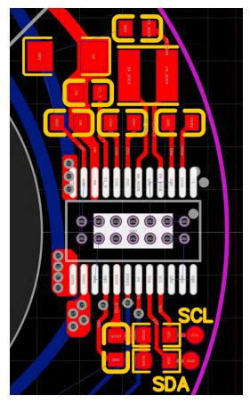
Figure 3-2. MCF8315 Layout Design Reference
