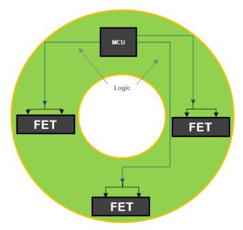
Figure 2-2. MCU+Pre-driver and External FET Architecture in Fan Application
