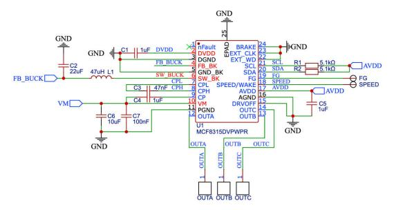
Figure 3-1. MCF8315 Schematic Design Reference
