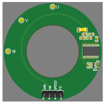
Figure 3-8. MCF8315 Simplifies Peripheral Design Layout 3D Picture
