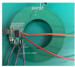
Figure 3-11. MCF8315 Single Layer With Inductance Version PCB
