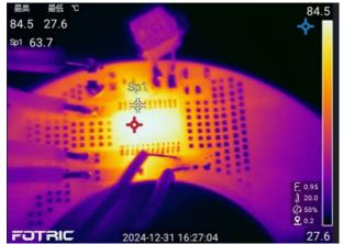
Figure 3-12. MCF8315 Single Layer With Inductance 20W Thermal Test Result
