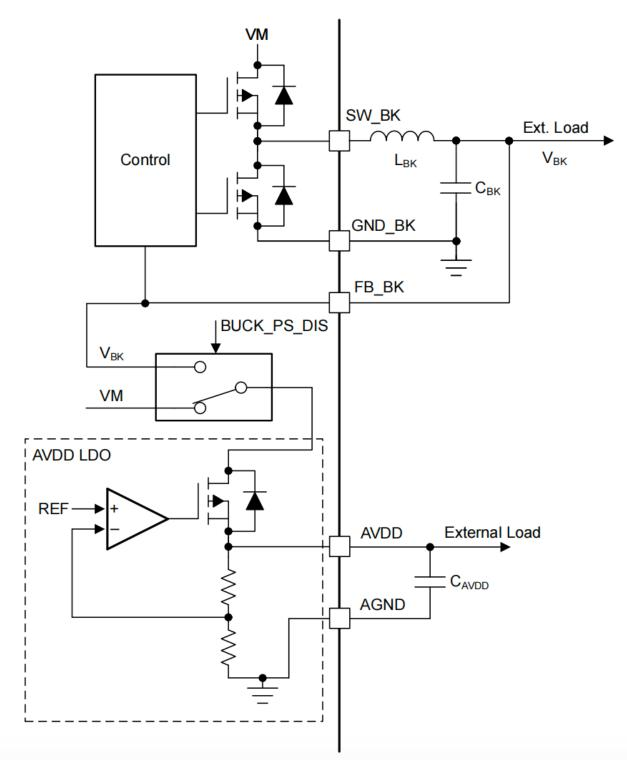
Figure 3-4. MCF8315 Power Sequence
