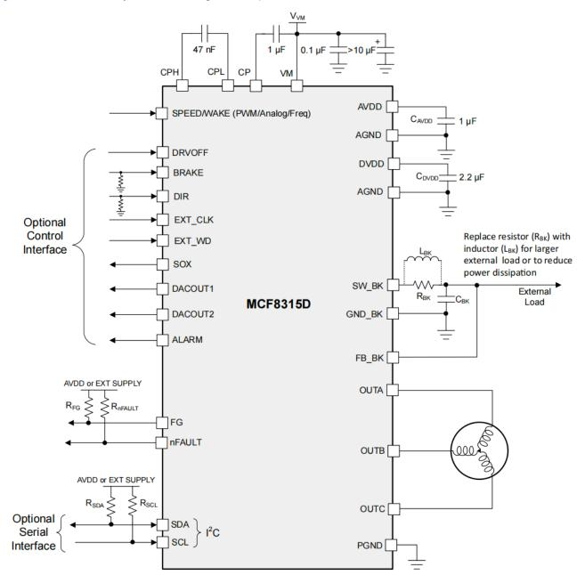
Figure 1-1. MCF8315 Block Diagram
