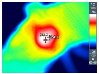
Figure 3-10. MCF8315 Two Layer With Inductance 30W Thermal Test Result
