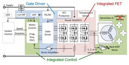
Figure 2-3. All in One Design Architecture in Fan Application
