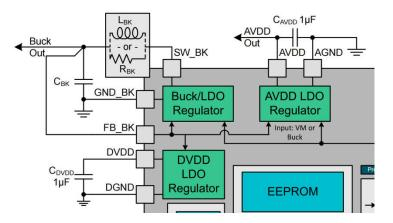
Figure 3-5. MCF8315 Power Rail
