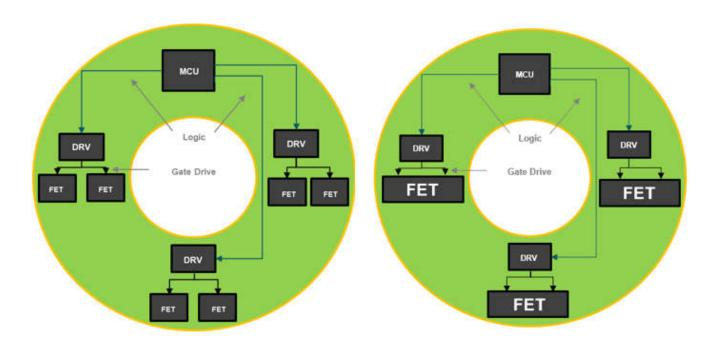
Figure 2-1. Discrete Hardware Design Architecture in Fan Application
