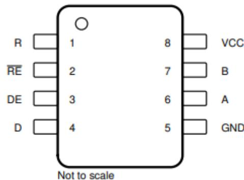
**Figure 3-2. Standard Pinout for 8-Pin Half Duplex RS-485 Transceivers**
