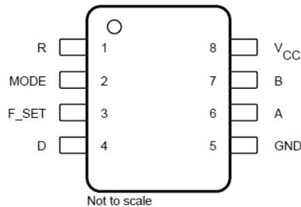
**Figure 3-1. Powerbus Standard Pinout**
