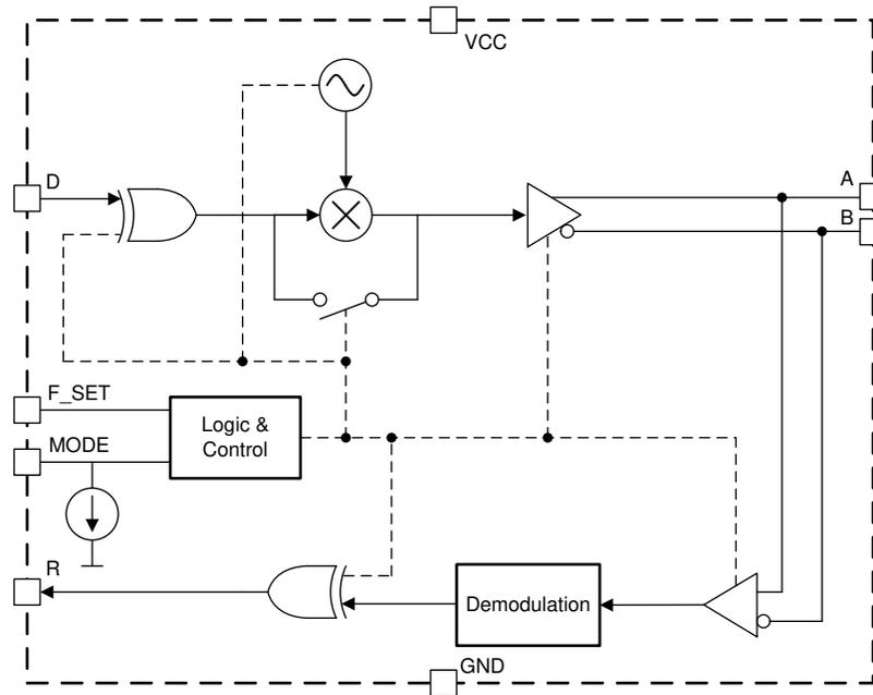
Figure 2-3. THVD80x0: Functional Block Diagram
