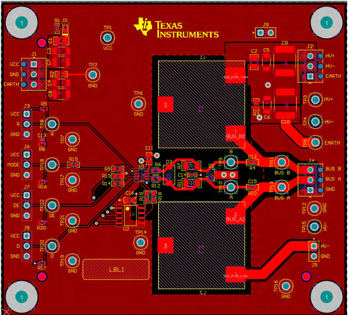
Figure 4-4. Example Layout - Top Layer
