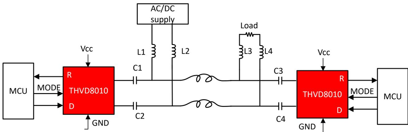
Figure 2-4. THVD80X0 Simplified Schematic (THVD8010 Shown)
