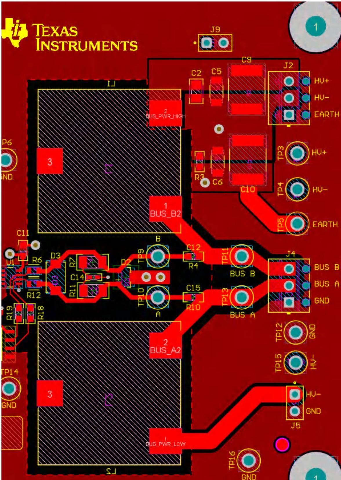
Figure 4-5. Close Up of Layout for IC PWR, IOs, Differential Bus, and High Power Interface
