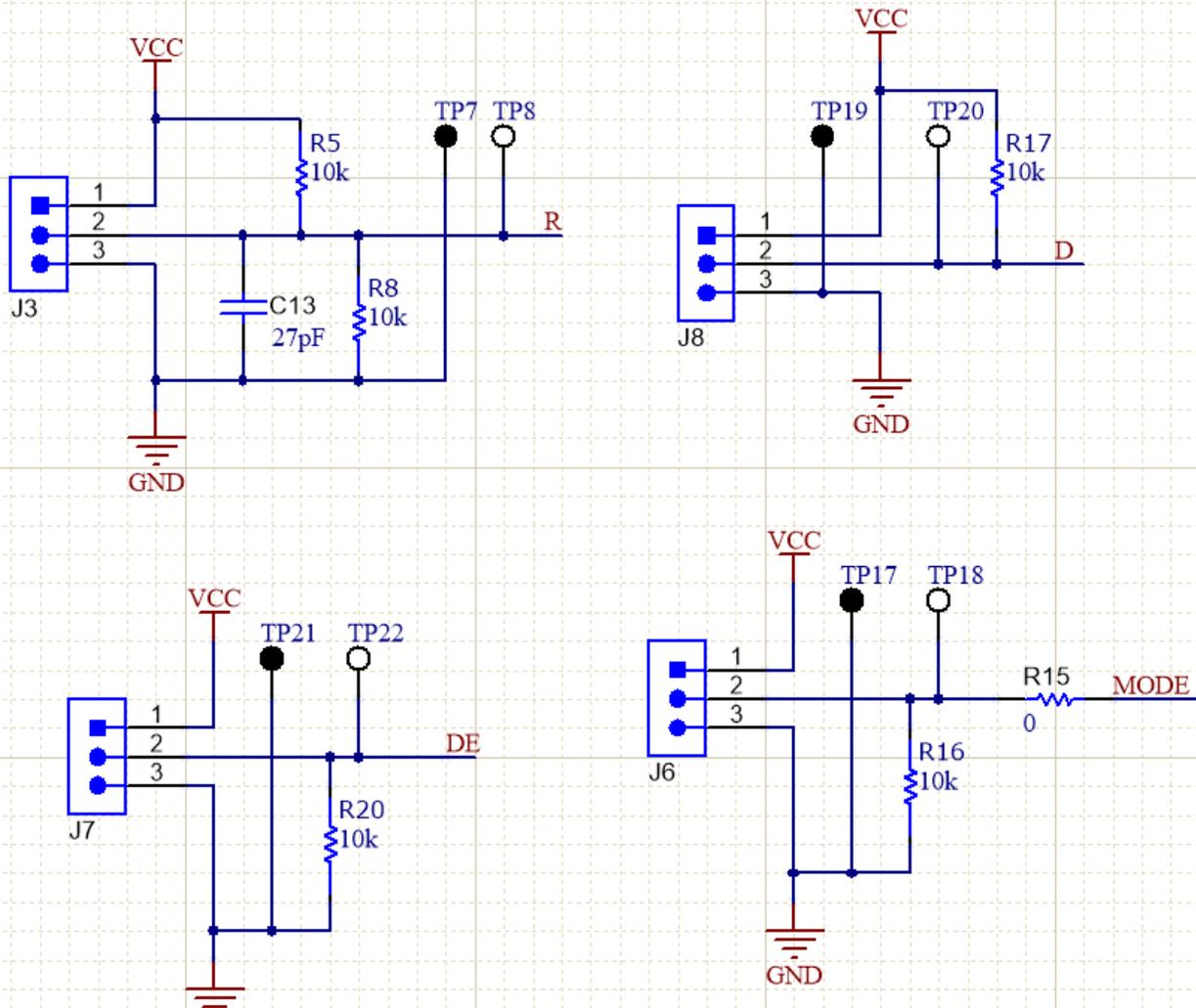
Figure 4-2. Generalized Single Ended I/O Schematic
