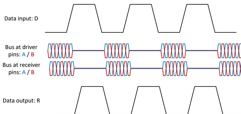
**Figure 2-1. THVD80x0: Modulation and Demodulation**
