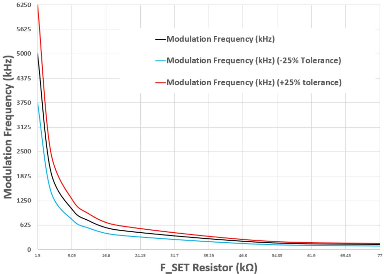
**Figure 2-2. THVD8000 Modulation Frequency v. Setting Resistor Value**
