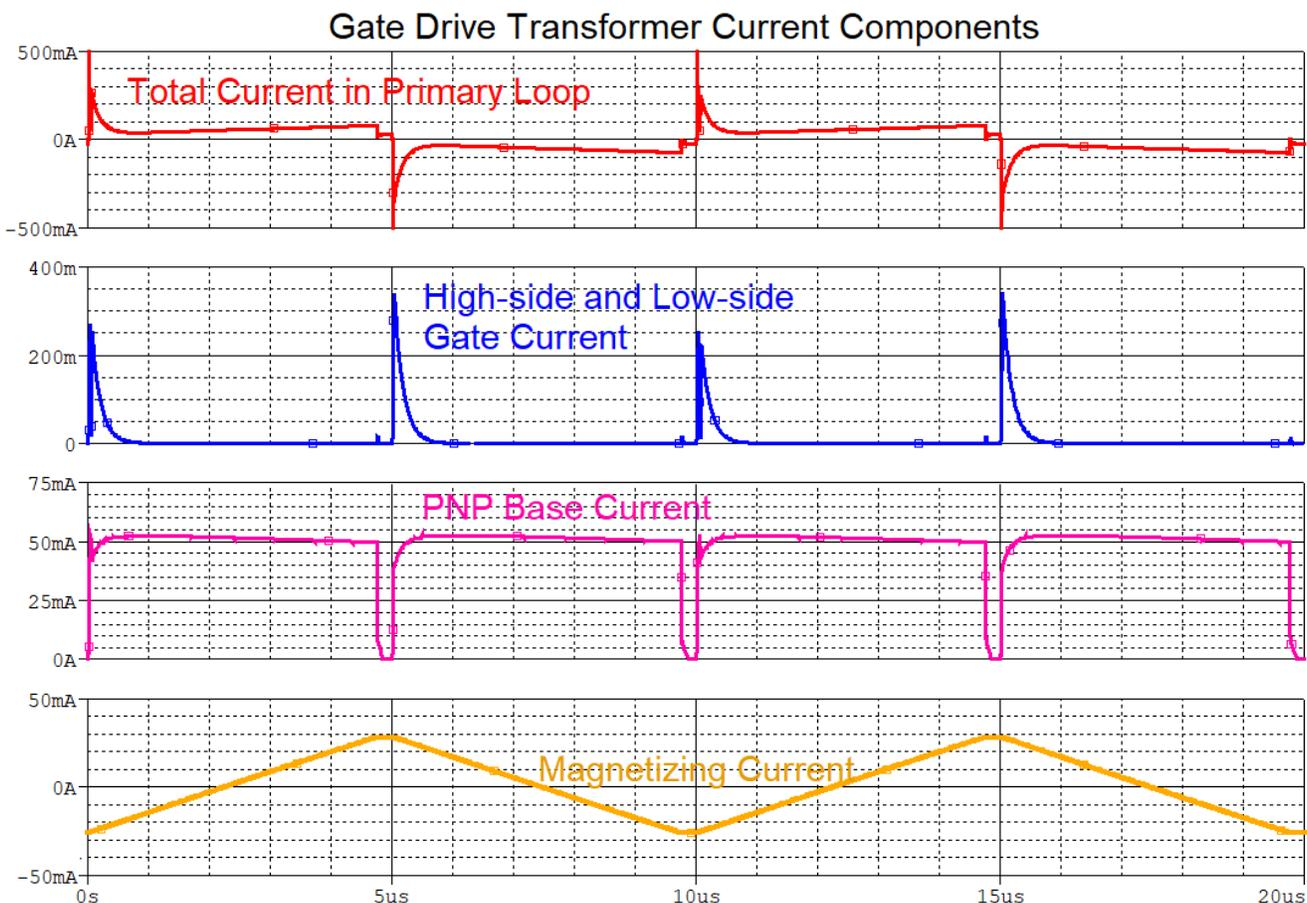
**Figure 4-1. Simulation Showing the Major Current Components in the Gate Drive Circuit**
