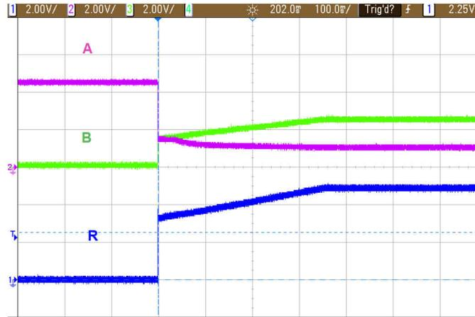
**Figure 2-9. SN65HVD888 Powered Up with Mis-wiring and Driver On**
