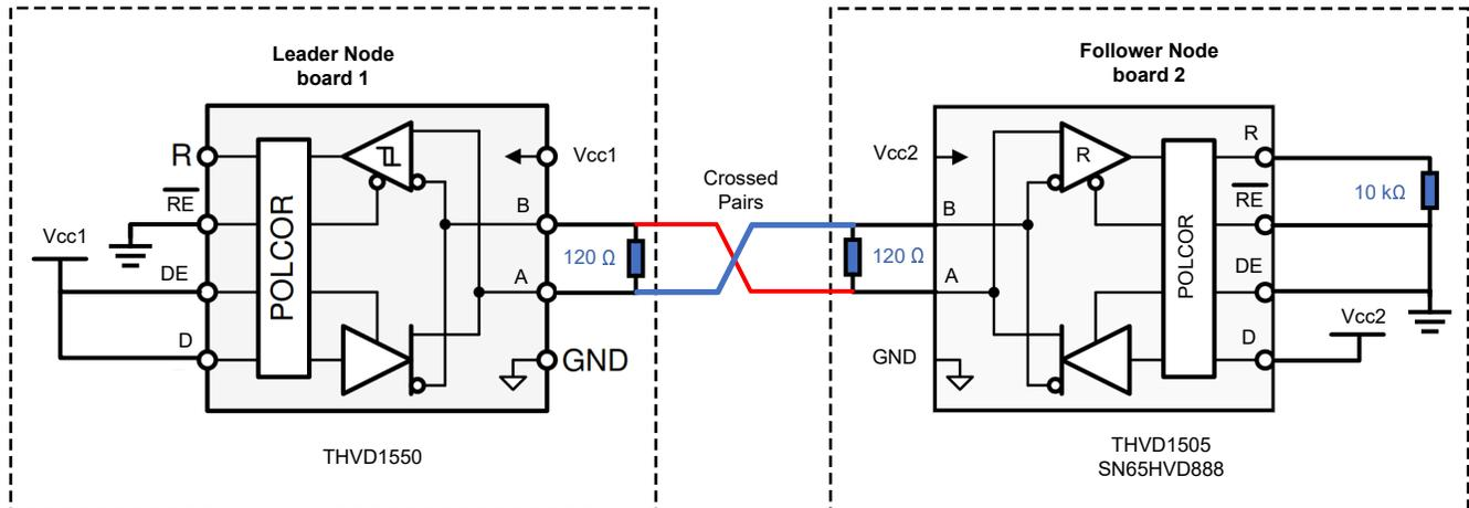
Figure 2-4. Test Case 2 Setup
