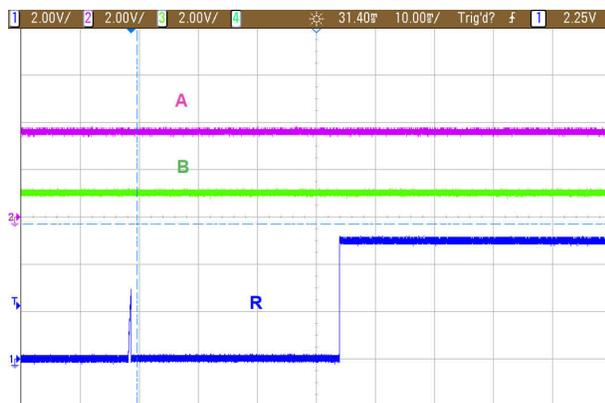
Figure 2-5. THVD1505 Powered Up with Mis-wiring
