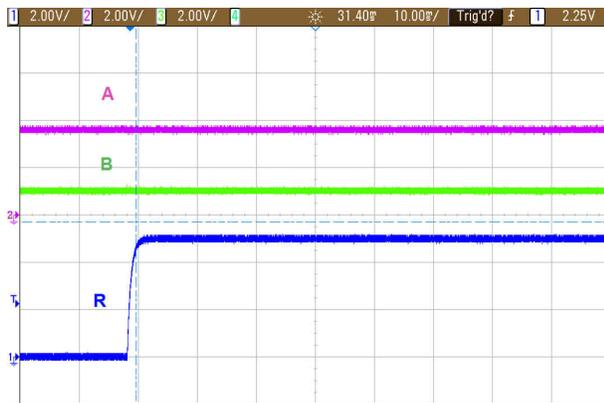
Figure 2-2. THVD1505 Powered Up with Correct Wiring
