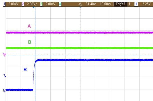
Figure 2-3. SN65HVD888 Powered Up with Correct Wiring
