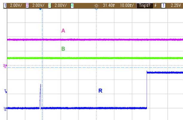
Figure 2-6. SN65HVD888 Powered Up with Mis-wiring
