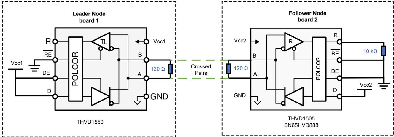
Figure 2-1. Test Case 1 Setup
