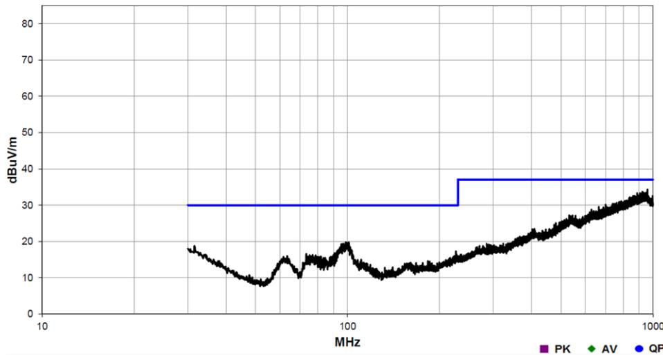
**Figure 3-7. Horizontal Radiated Emissions Measurements per CISPR32 Class B for PH9085.011NL with 1m Cable on Isolated GND and 22Ω, 820pF Snubber**
