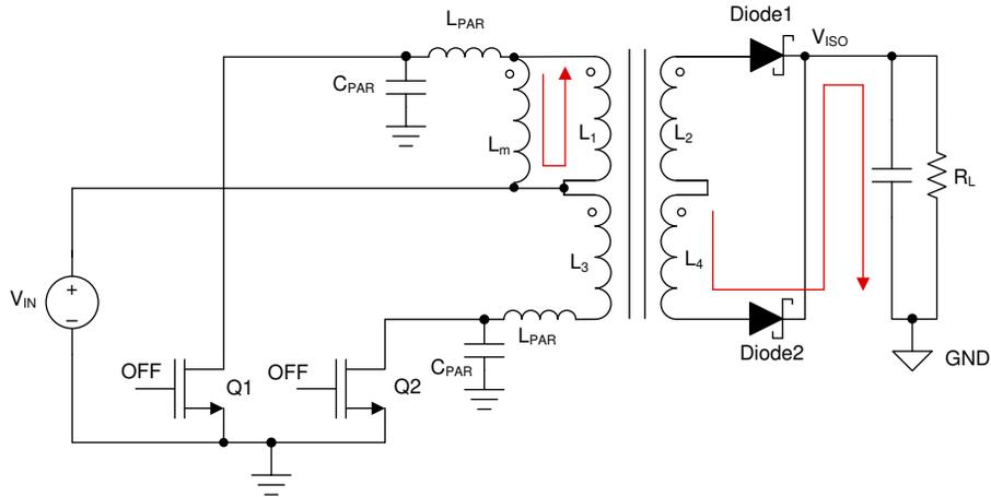
**Figure 1-2. Push-pull Isolated Power Supply with Switching Parasitics Create a Ringing LC Network**
