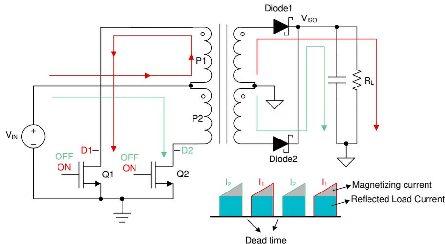
**Figure 1-1. Complementary Energy Transmission by Push-pull Power Supplies**
