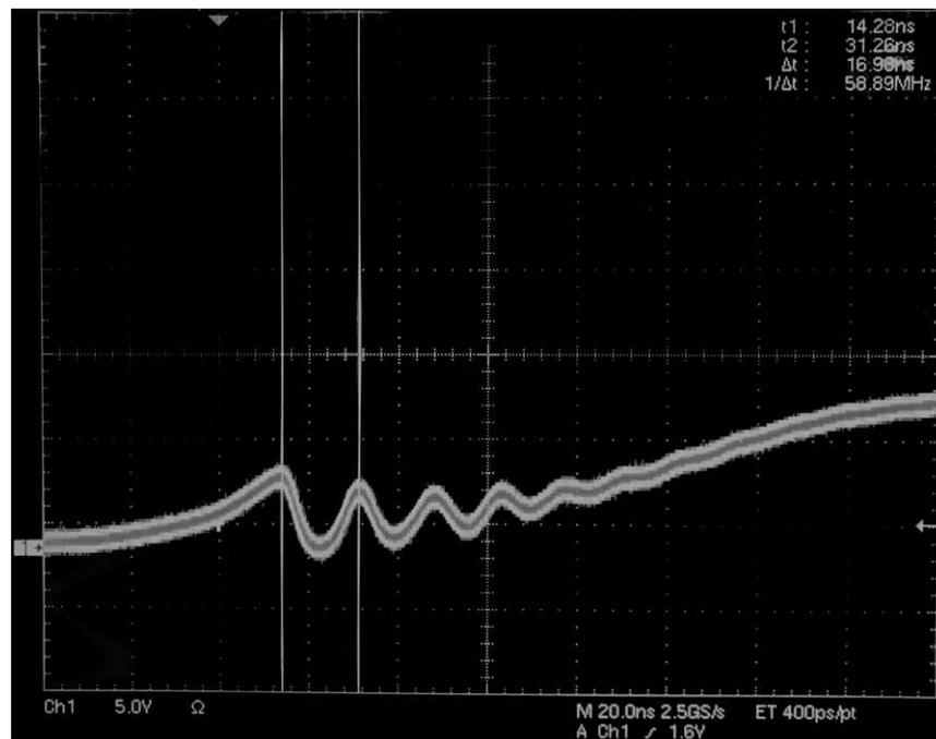
**Figure 3-2. PH9085.011NL Time Domain D1/D2 Infinite Persistence Waveform without RC Snubber**
