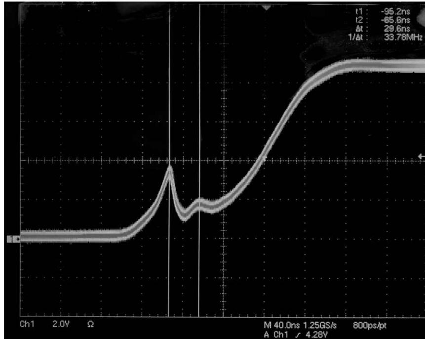
Figure 3-3. PH9085.011NL Time Domain D1/D2 Infinite Persistence Waveform with 22Ω, 820pF Snubber
