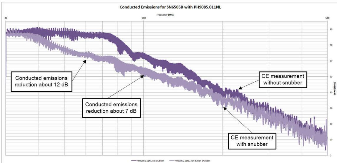
Figure 3-4. Conducted Emissions Comparison With and Without Snubber for this PCB with PH9085.011NL
