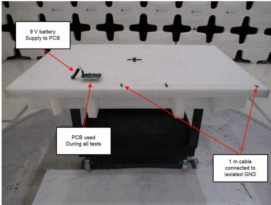
**Figure 3-5. Radiated Emissions Test Environment per CISPR32**
