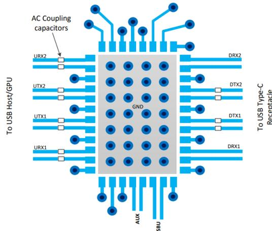
**Figure 4. AC-Coupling Capacitor Layout Symmetry Example**
