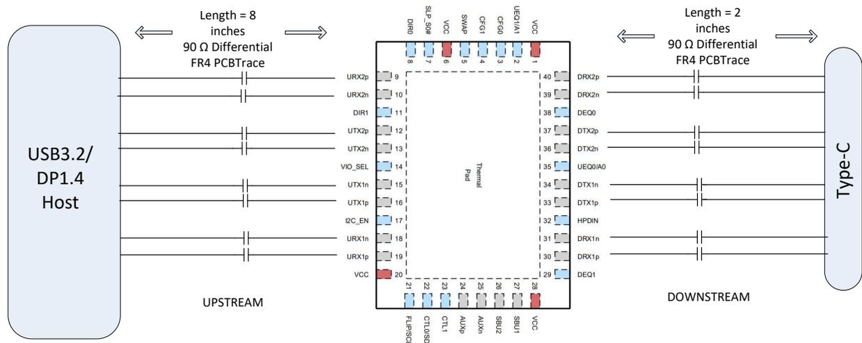
Using the given trace lengths and data rate in this example, the method to select the equalization values for Upstream and Downstream EQ is to select the closest EQ gain value available to match the trace loss as follows.
