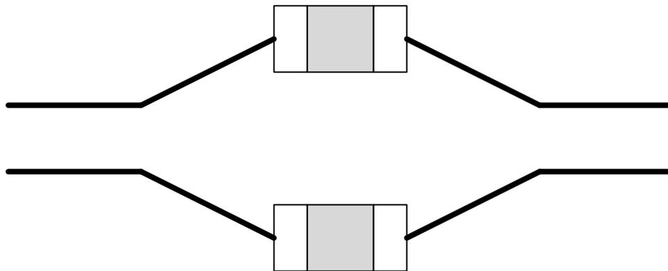
**NOTE:** Adding test points to the high-speed traces can cause impedance discontinuity which negatively impacts signal performance. If test points are used, they should be placed in series and symmetrically. They must not be placed in a manner that causes a stub on the transmission line.
