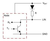
Figure 3-1. Simplified LIN Driver Schematic
