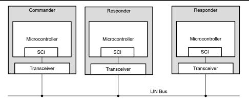
Figure 2-1. High-Level LIN Transceiver in Network
