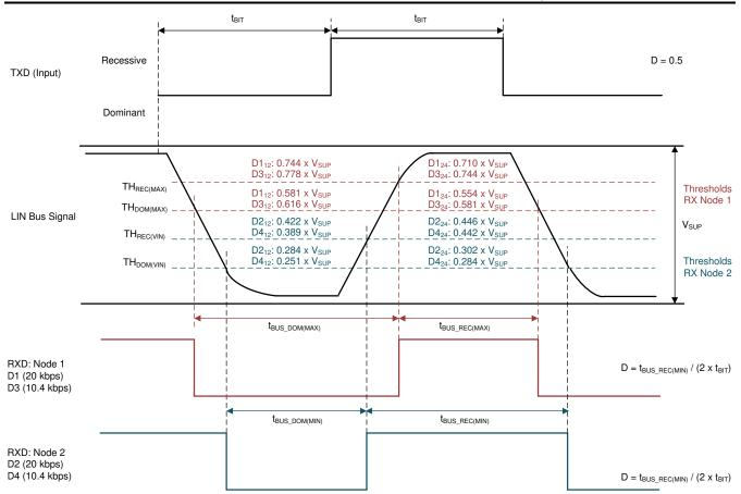
Figure 3-5. Bus Duty Cycle Requirement
