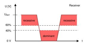
Figure 3-3. Bus Signal Thresholds for Receivers
