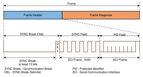
Figure 2-2. LIN Frame Header Explanation
