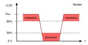
Figure 3-2. Bus Signal Thresholds for Senders
