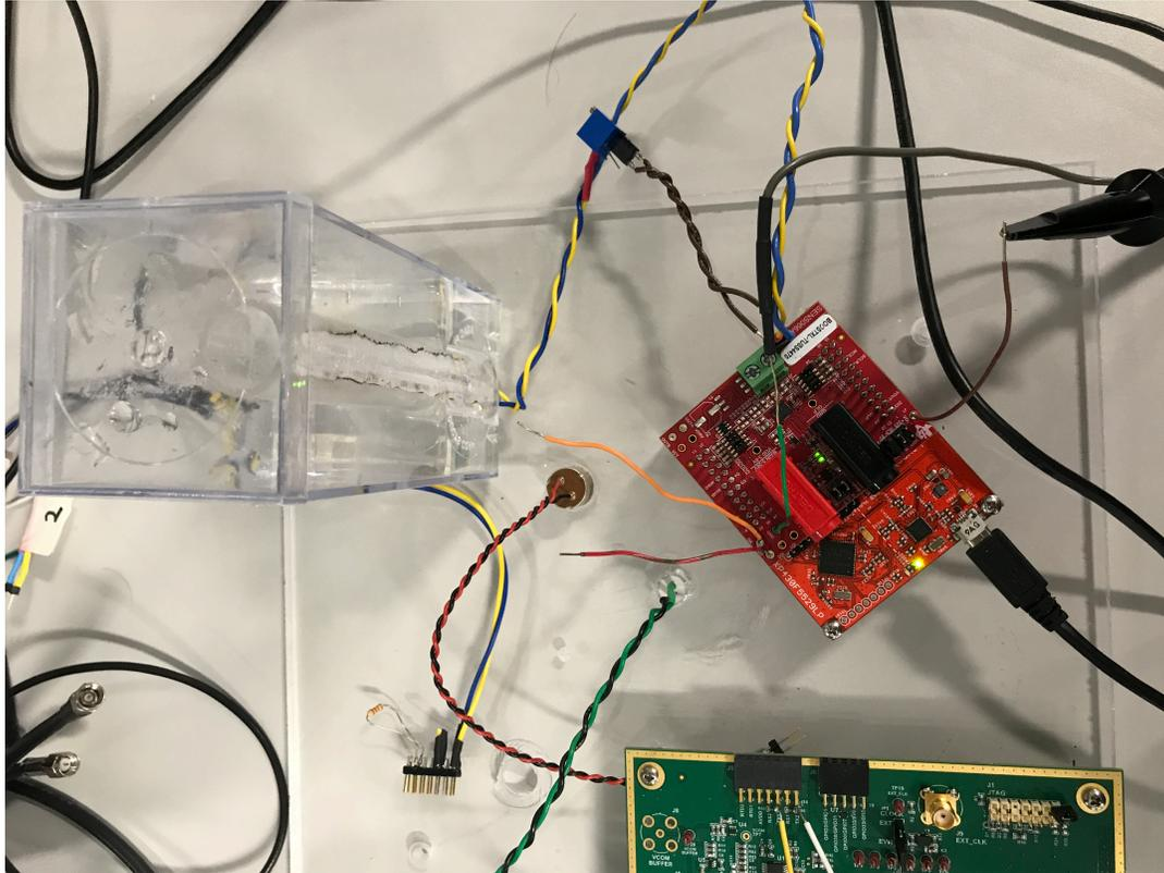
**Figure 2-3. Short-Range Water-Coupled Level Sensing Test Environment**
