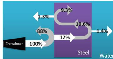
**Figure 1-1. Reflection Coefficients for Water and Steel Boundaries**
