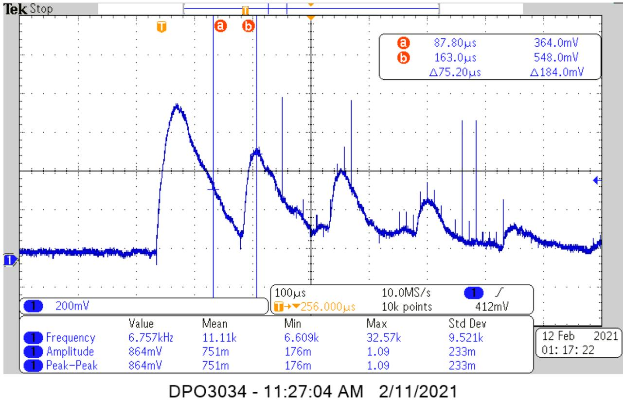
Figure 6-2. TUSS4470 1 MHz Water Level Measurement: 500Ω damping
