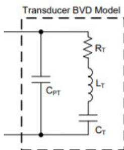
Figure 1-3. Transducer BVD Model
