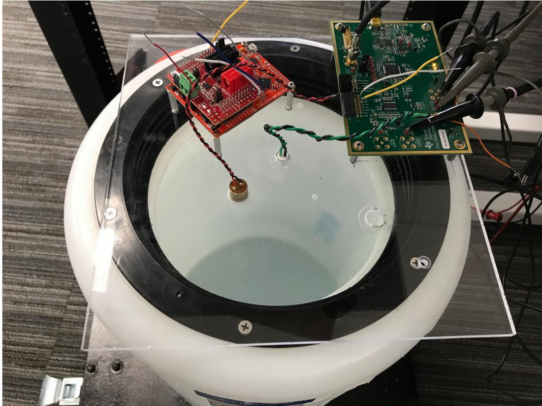
**Figure 2-1. Short Range Air-Coupled Level Sensing Test Environment**
