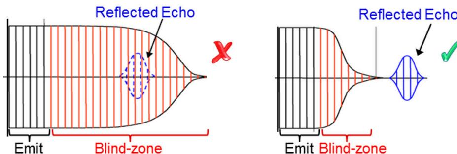
Figure 1-4. Monostatic Ring Decay
