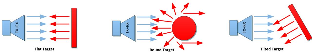
**Figure 1-2. Target Geometry Impact**
