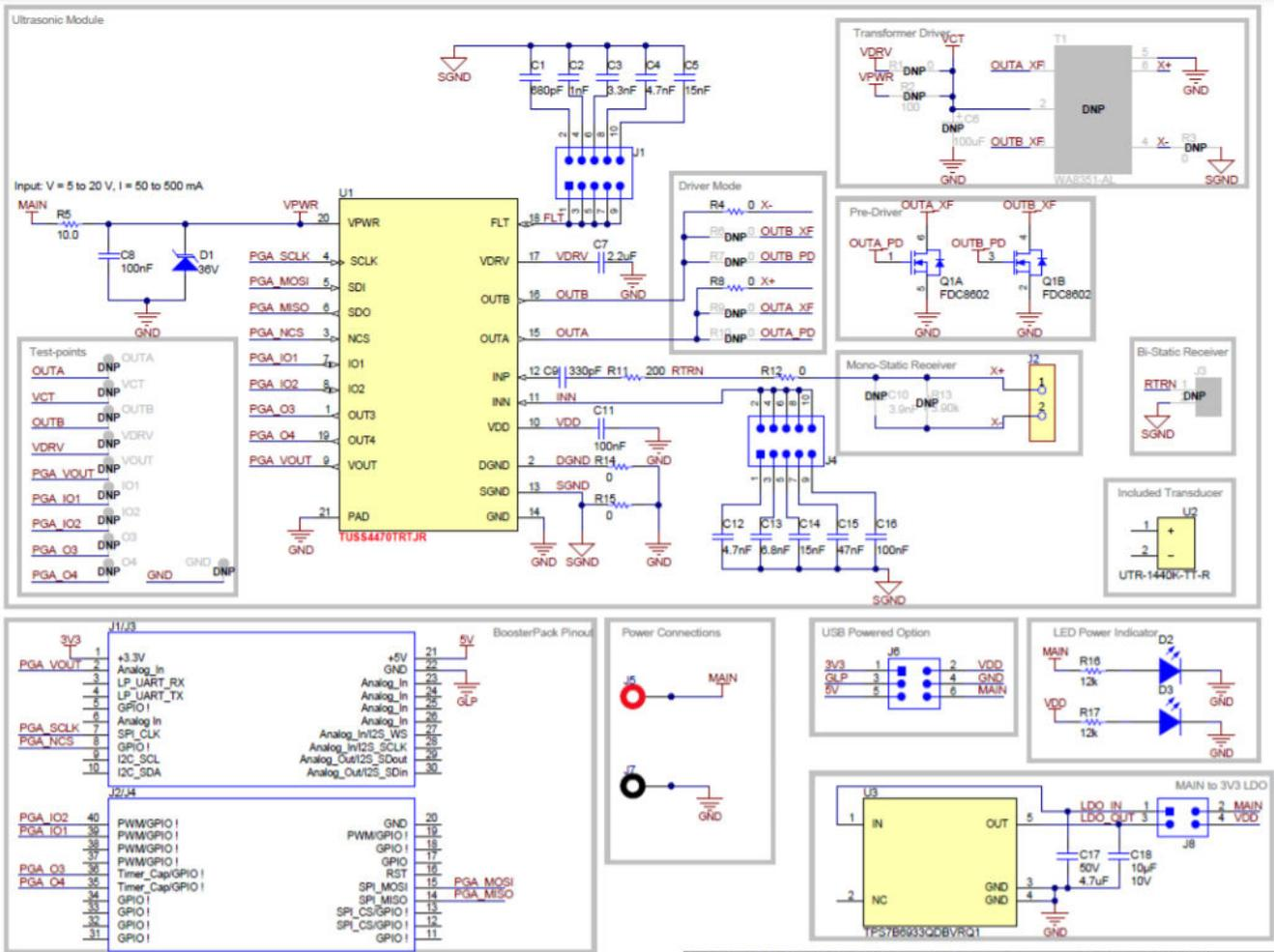
Figure A-3. BOOSTXL-TUSS4470 Schematic
