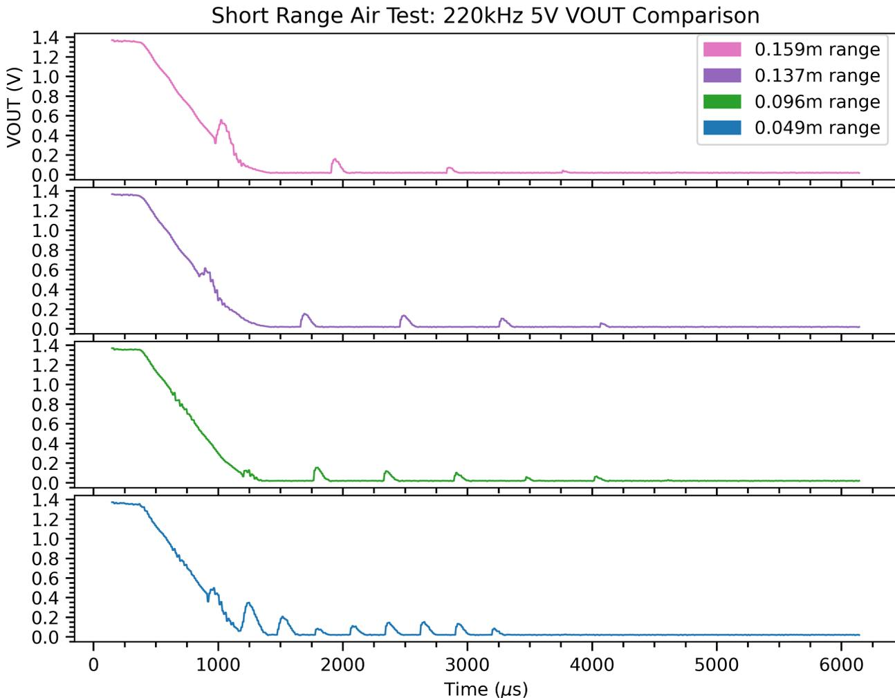
**Figure 3-1. Short Range Air-Coupled Results: TUSS4470**
