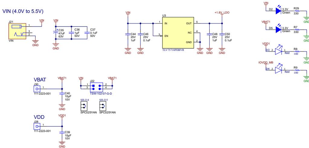
Figure 5-4. TAS2118EVM Schematic (Sheet 4 of 4)
