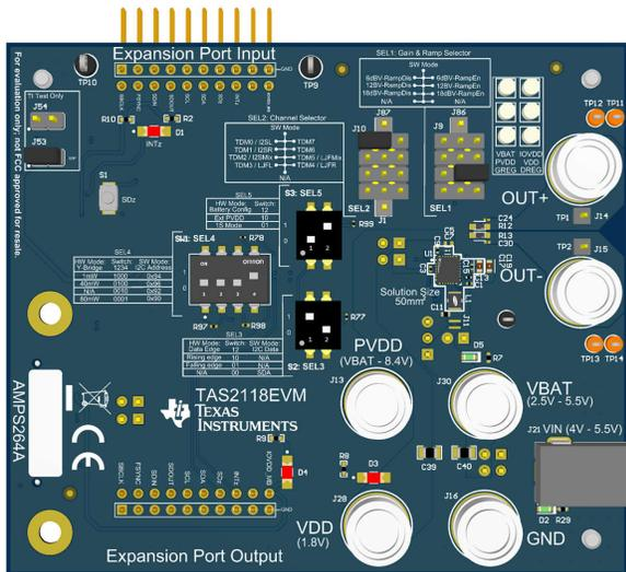
Figure 2-6. Hardware Pin-Control Mode Jumper Settings (Front Side)
