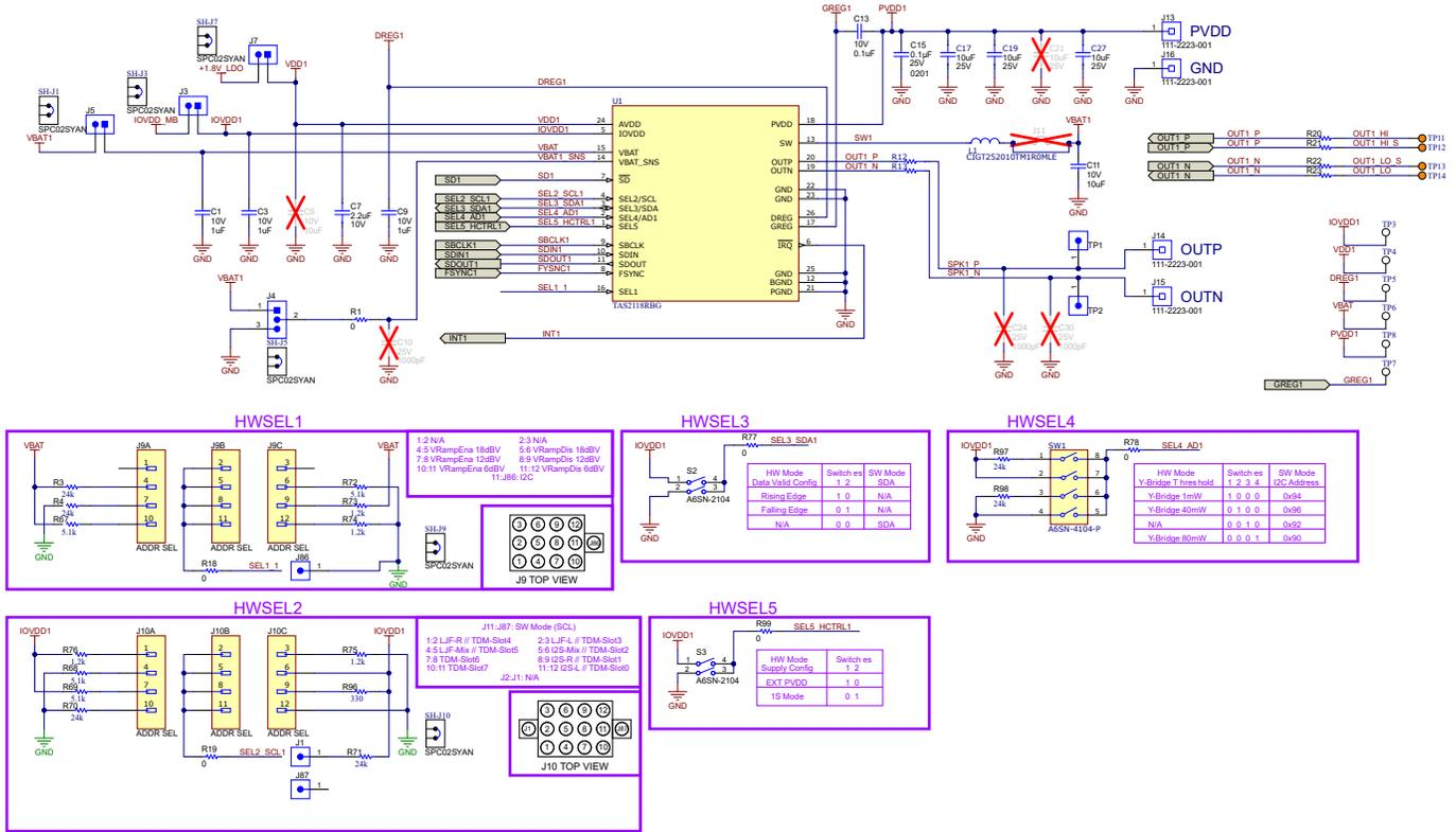
Figure 5-1. TAS2118EVM Schematic (Sheet 1 of 4)
