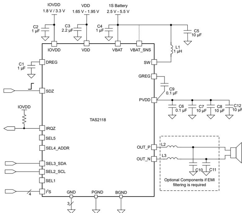
**Figure 1-1. Application Diagram for 1S Battery System**
