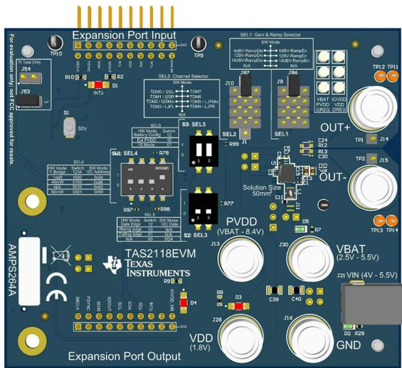
**Figure 2-1. Software Mode Jumper Settings (Front Side)**
