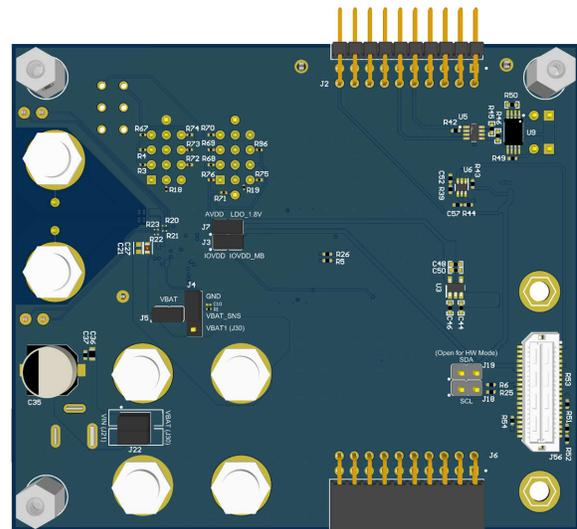
Figure 2-7. Hardware Pin-Control Mode Jumper Settings (Back Side)
