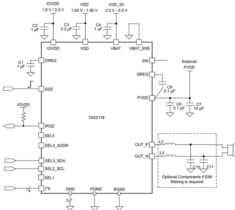
**Figure 1-2. Application Diagram for External PVDD System**
