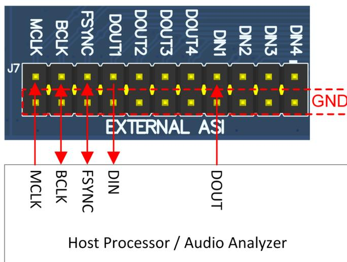
Figure 3-5. AC-MB Connection with External Audio Serial Interface
