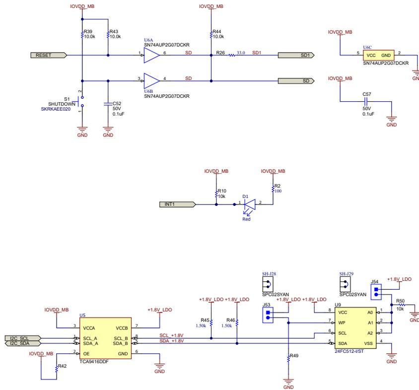
Figure 5-3. TAS2118EVM Schematic (Sheet 3 of 4)
