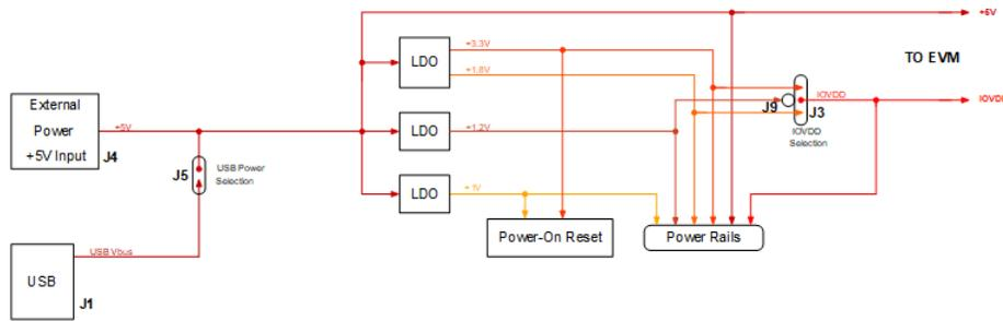
Figure 3-6. Power -Supply Distribution of the AC-MB
