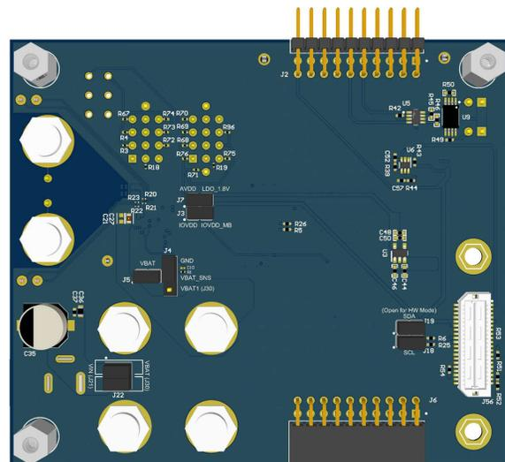
**Figure 2-2. Software Mode Jumper Settings (Back Side)**
