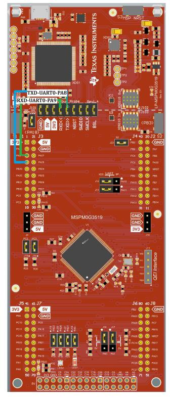
Figure 2-6. LP-MSPM0G3519 Backchannel Connection to UART0
