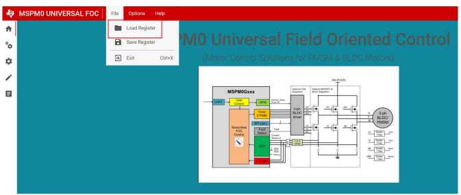
Figure 4-8. Option to Load Register Configurations
