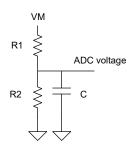
Figure 2-3. ADC Voltage Divider
