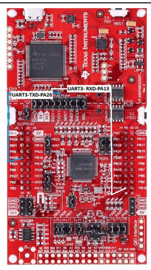
Figure 2-5. LP-MSPM0G3507 Backchannel Connection to UART3
