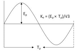
Figure 6-5. BEMF Constant Measurement
