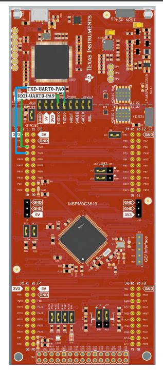
Figure 2-6. LP-MSPM0G3519 Backchannel Connection to UART0
