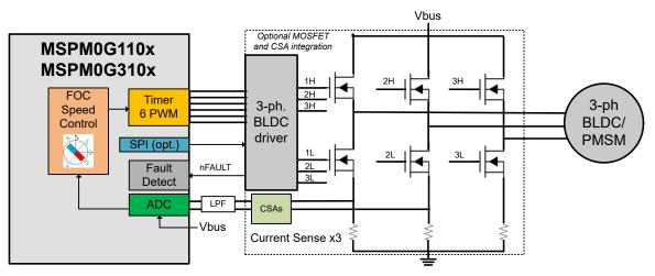
Figure 1-1. Simplified Schematic of MSPM0Gxxx + BLDC Motor Driver
