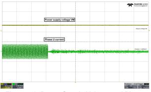
Figure 7-3. Power Supply Voltage and Phase Current Waveform When AVS is Enabled
