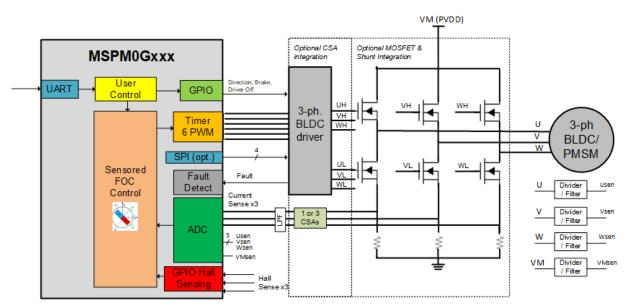
Figure 2-1. MSPM0Gxxx + BLDC Motor Driver - Sensored FOC Block Diagram
