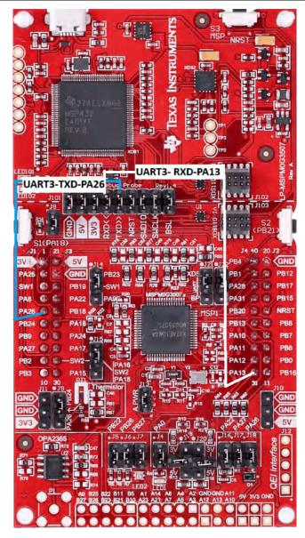
Figure 2-5. LP-MSPM0G3507 Backchannel Connection to UART3
