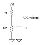
Figure 2-3. ADC Voltage Divider
