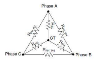
Figure 6-3. Resistance Measurement
