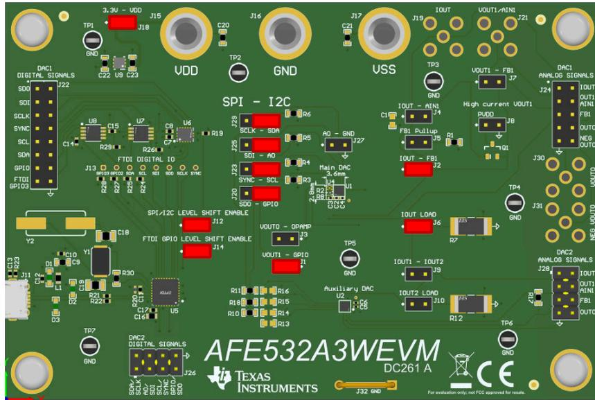
**Figure 2-5. AFE532A3WEVM Comparator Input Jumper Settings**
