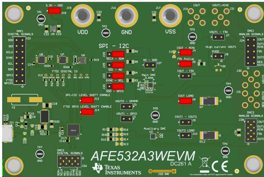
**Figure 2-6. AFE532A3WEVM ADC Input Jumper Settings**
