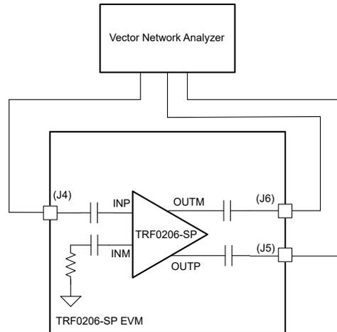
**Figure 3-1. S-Parameter Test Setup**
