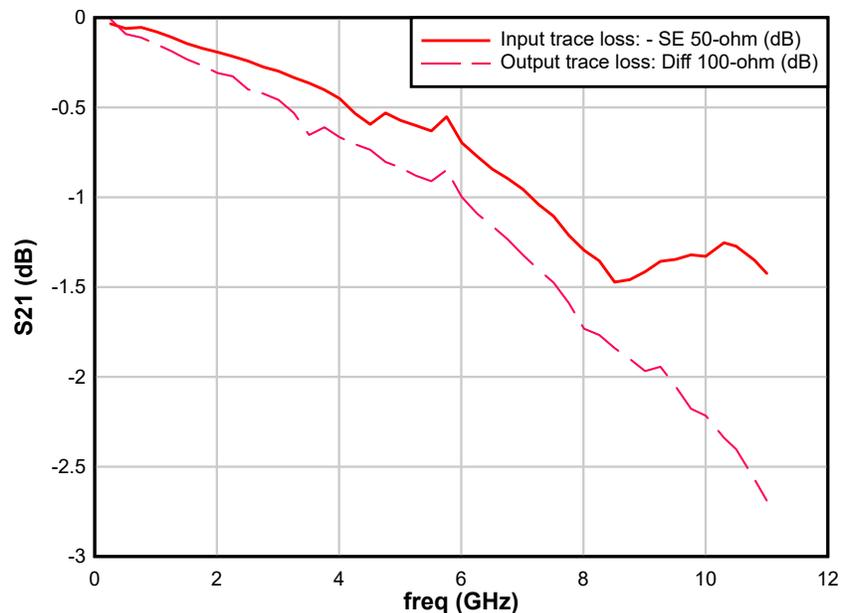
**Figure 3-2. PCB Trace Loss vs Frequency**
