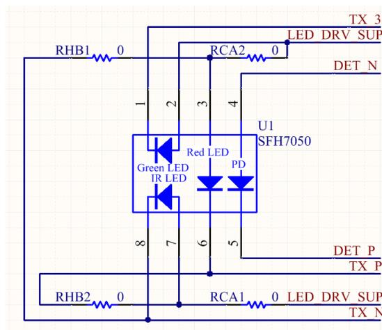
**Figure 43. OSRAM SFH7050 Sensor Board LED Connections**
