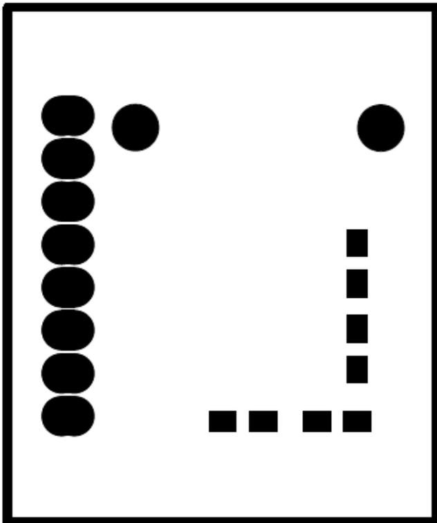
Figure 77. SFH7050 Sensor Board Bottom Solder Mask
