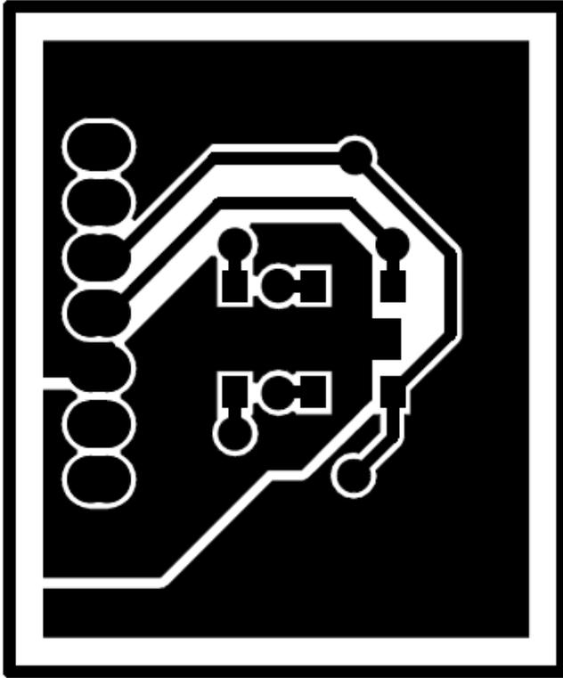
Figure 81. NJL5310R Sensor Board Top Copper
