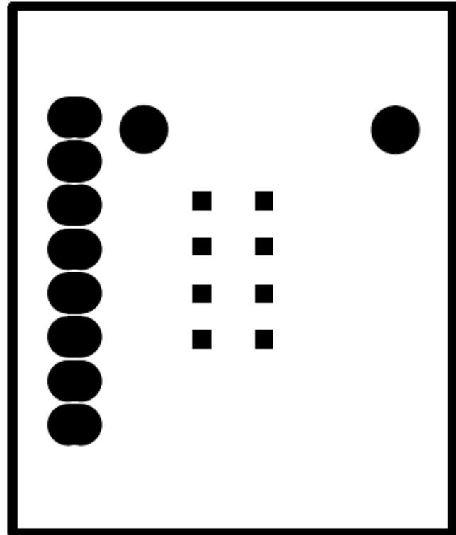
Figure 74. SFH7050 Sensor Board Top Solder Mask
