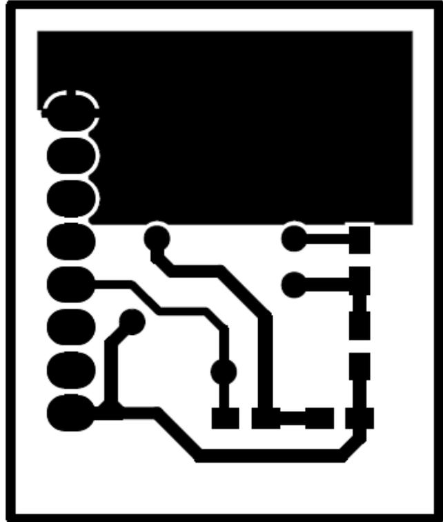
Figure 76. SFH7050 Sensor Board Bottom Copper
