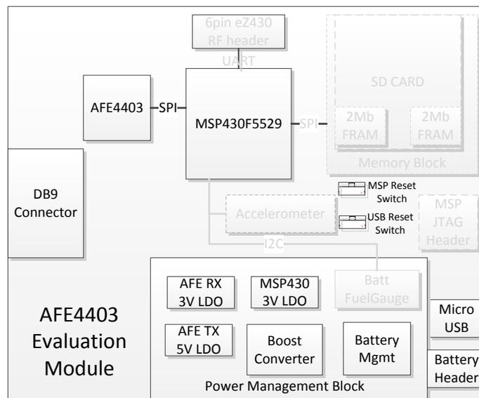
**Figure 31. AFE4403EVM Block Diagram**
