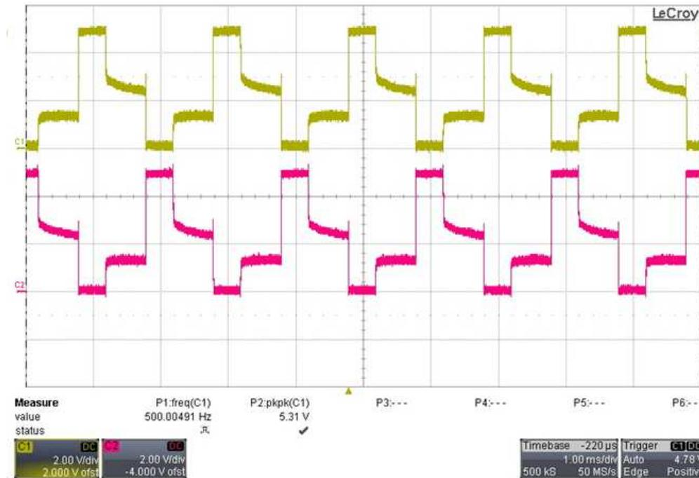
Figure 48. TXP and TXN Without Pulse Oximeter Cable
