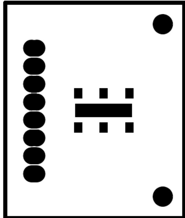
Figure 80. NJL5310R Sensor Board Top Solder Mask
