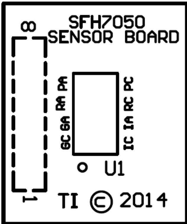
Figure 73. SFH7050 Sensor Board Top Silk Screen
