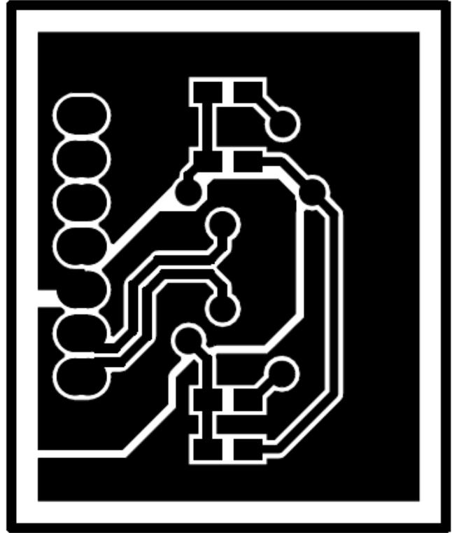
Figure 82. NJL5310R Sensor Board Bottom Copper
