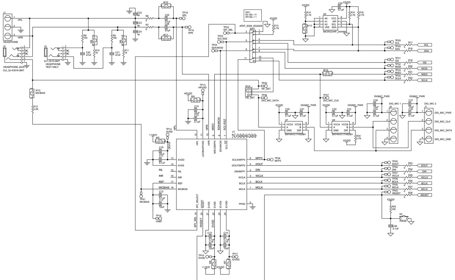
Figure 10. TLV320DAC3253EVM Schematic (Sheet 1 of 2)
