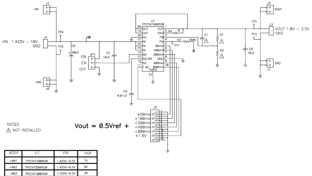
Figure 6. TPS7A7x00EVM-718 Schematic
