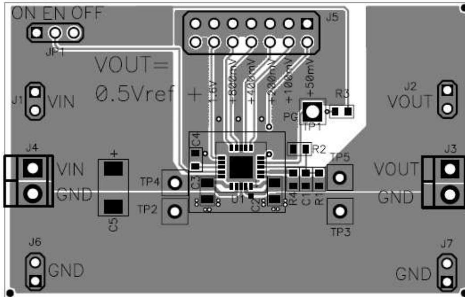
Figure 3. Assembly Layer
