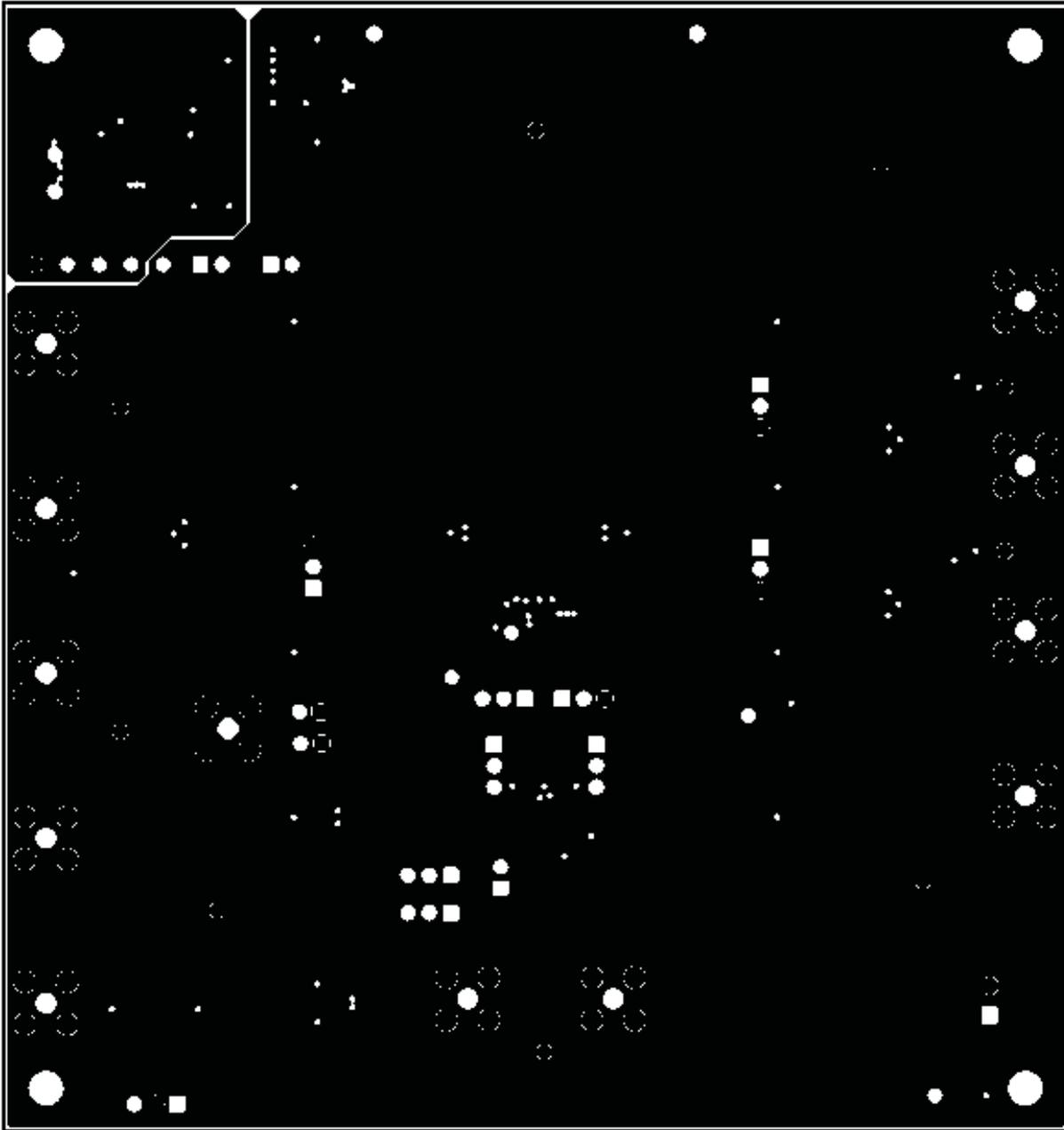
Figure 30. ADS5294EVM Internal Layer 4, Ground – Top View
