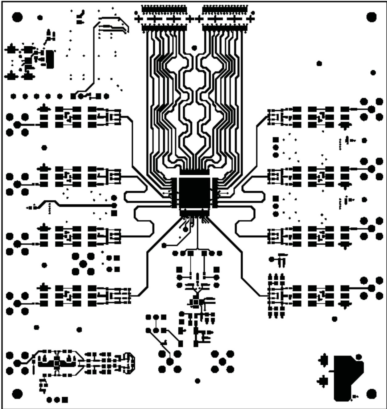
Figure 26. ADS5294EVM Top Layer Copper – Top View
