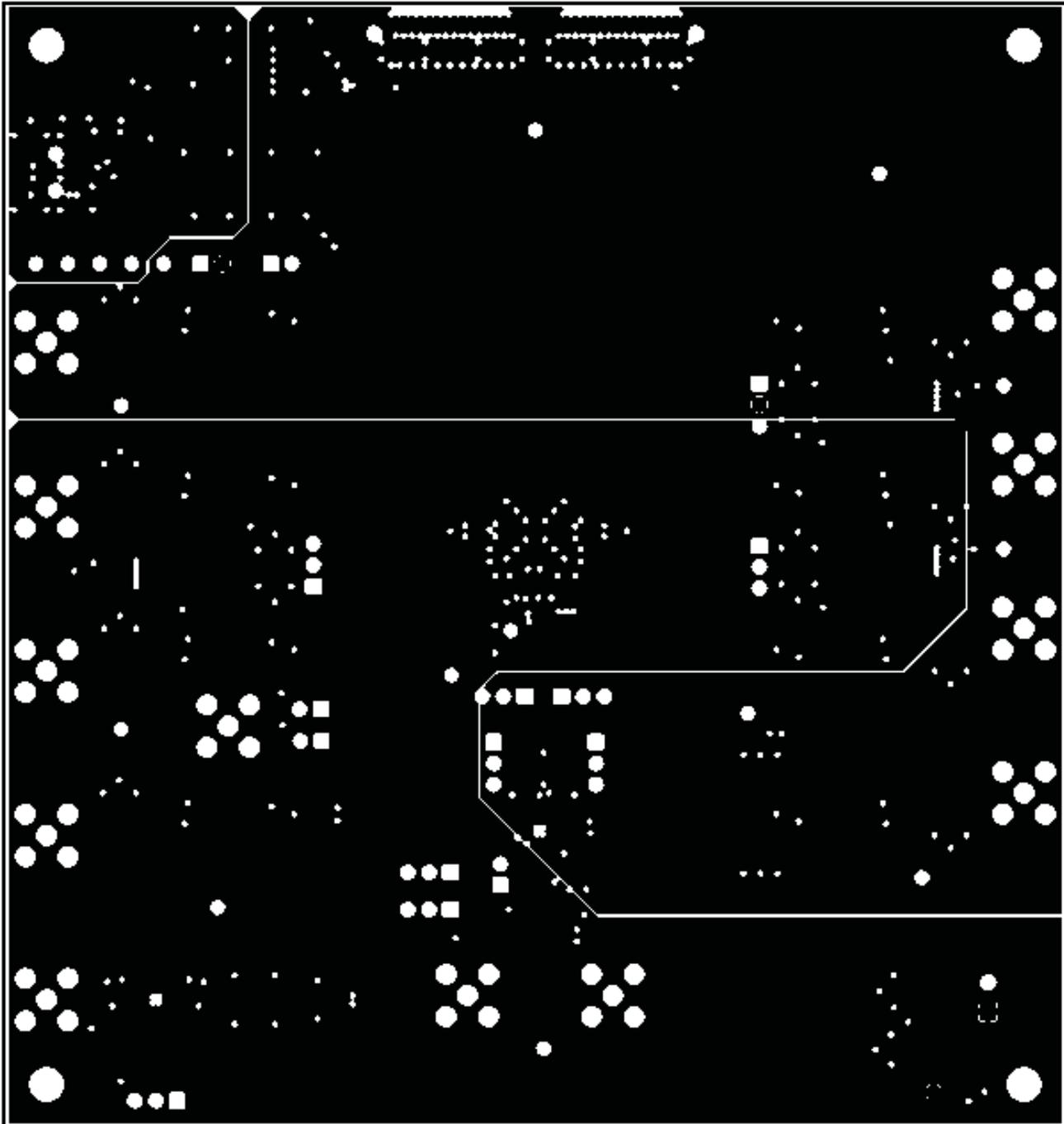
Figure 28. ADS5294EVM Internal Layer 2, Power – Top View
