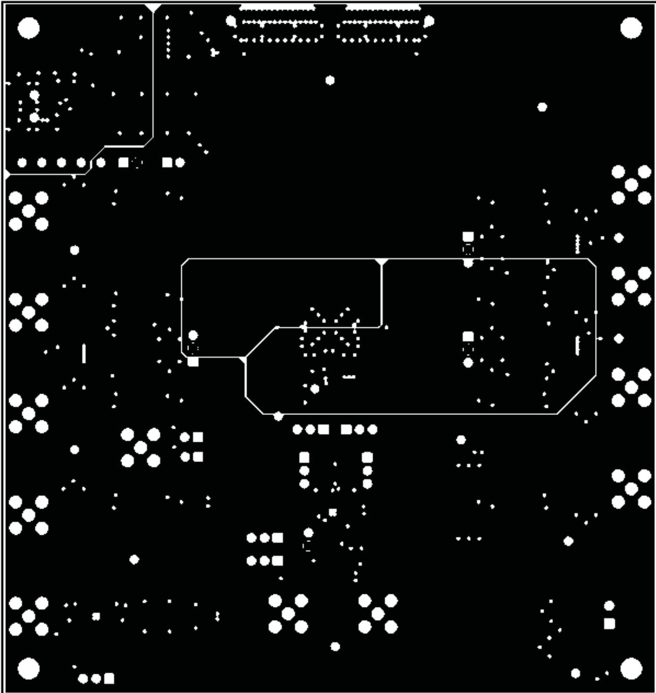
Figure 29. ADS5294EVM Internal Layer 3, Power – Top View
