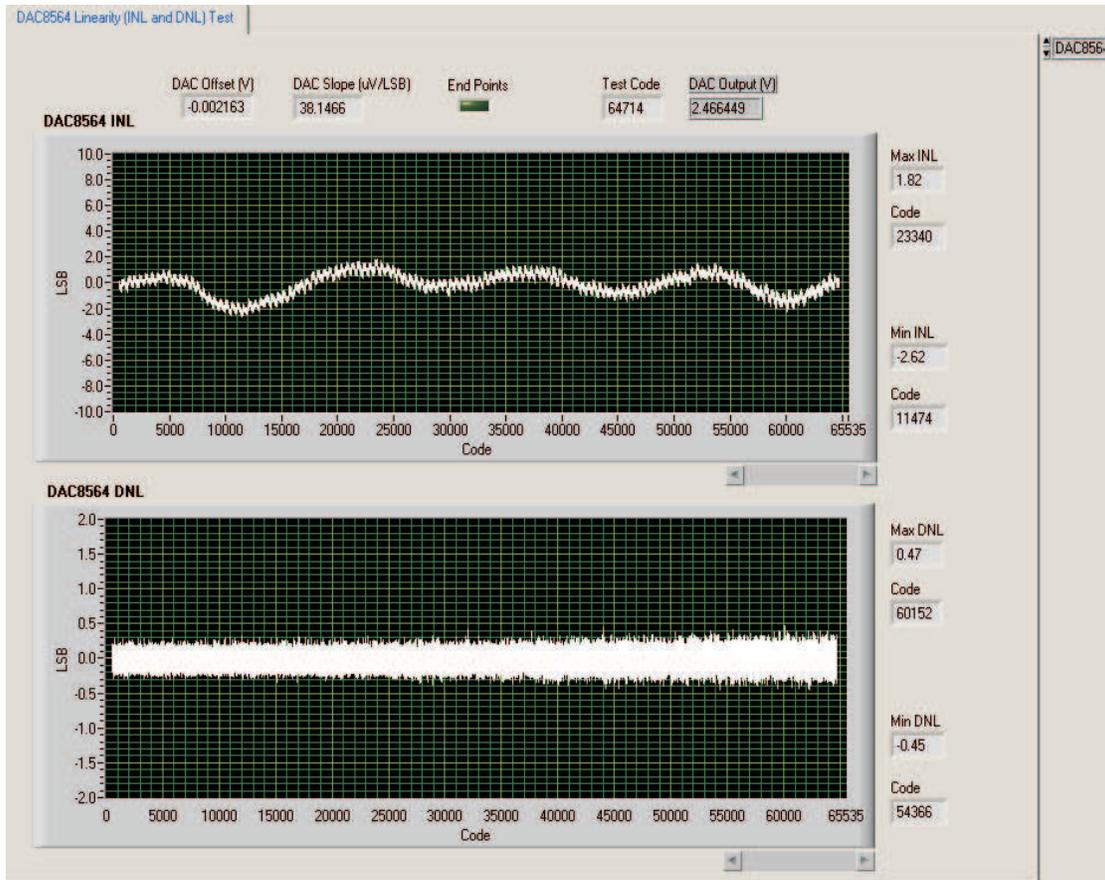
Figure 13. DAC8565 Channel A INL and DNL Characteristic Plot
