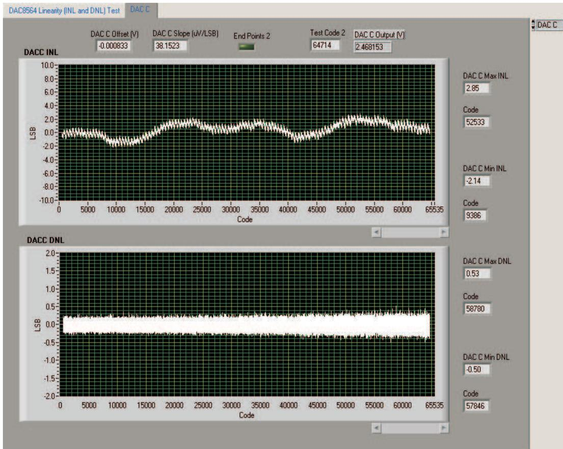
Figure 15. DAC8565 Channel C INL and DNL Characteristic Plot
