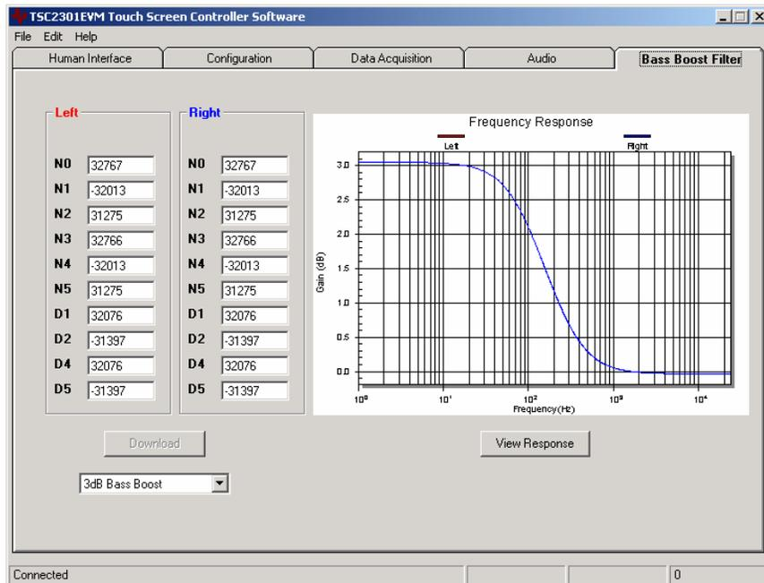
Different filter coefficients can be loaded for left and right channels, though usually these are set the same. Three *preconfigured* filters are selectable using the drop-down list box at the bottom of this screen. Selecting one of these updates the coefficients and causes the graph of the filter response to update. However, nothing is loaded into the TSC2301 until the *Download* button is pressed.
