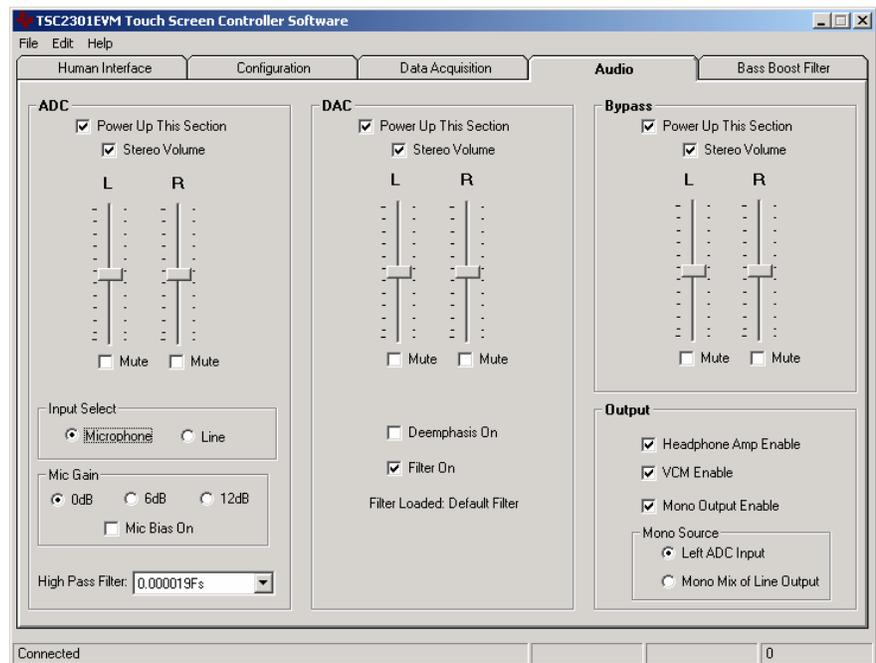
The microphone gain may be set to 0 dB, 6 dB, or 12 dB. A microphone bias voltage can also be generated by the TSC2301; checking the *Mic Bias On* checkbox enables this feature. Note that to use this feature, JMP4 must be set to positions 2-3.
