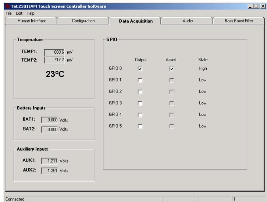
When on this screen, the TSC2301 is commanded to perform a PORT SCAN function, which updates the battery and auxiliary input voltage readings, and then is commanded to perform a TEMP1 and TEMP2 measurement. These measurements are all repeated once every second, and the results are displayed on this screen.
