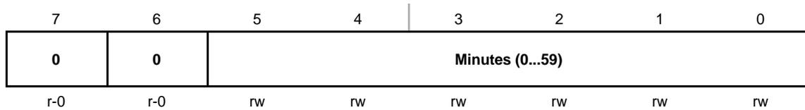
**RTCMIN, RTC Minutes Register, Calendar Mode with BCD Format**
