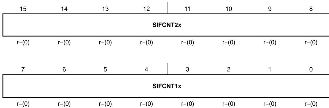
**SIFCNT2x** Bits 15-8 SIFCNT2. These bits are the SIFCNT2 counter. SIFCNT2 is reset when SIFEN = 0 or if read when SIFCNTRST = 1.
