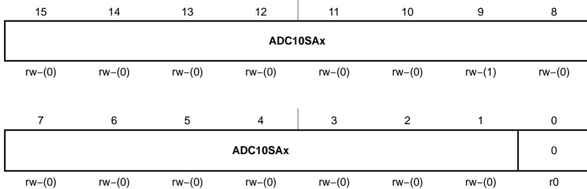
**ADC10SAx** Bits 15-1 ADC10 start address. These bits are the start address for the DTC. A write to register ADC10SA is required to initiate DTC transfers.
