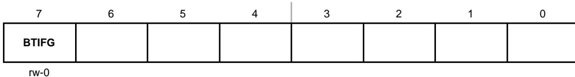
**BTIFG**      Bit 7      Basic Timer1 interrupt flag. Because other bits in IFG2 may be used for other modules, it is recommended to clear BTIFG automatically by servicing the interrupt, or by using `BIS.B` or `BIC.B` instructions, rather than `MOV.B` or `CLR.B` instructions.
