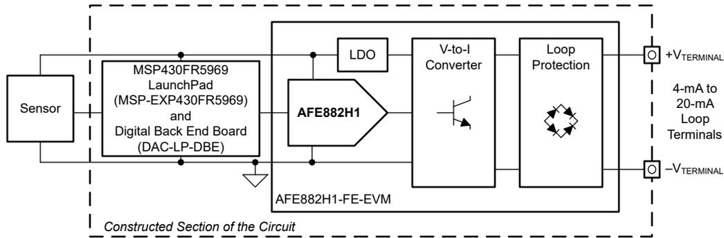
**Figure 2-5. Block Diagram of a 2-wire Transmitter Design Using an AFE882H1 Evaluation Module and a Digital-Back-End Board**
