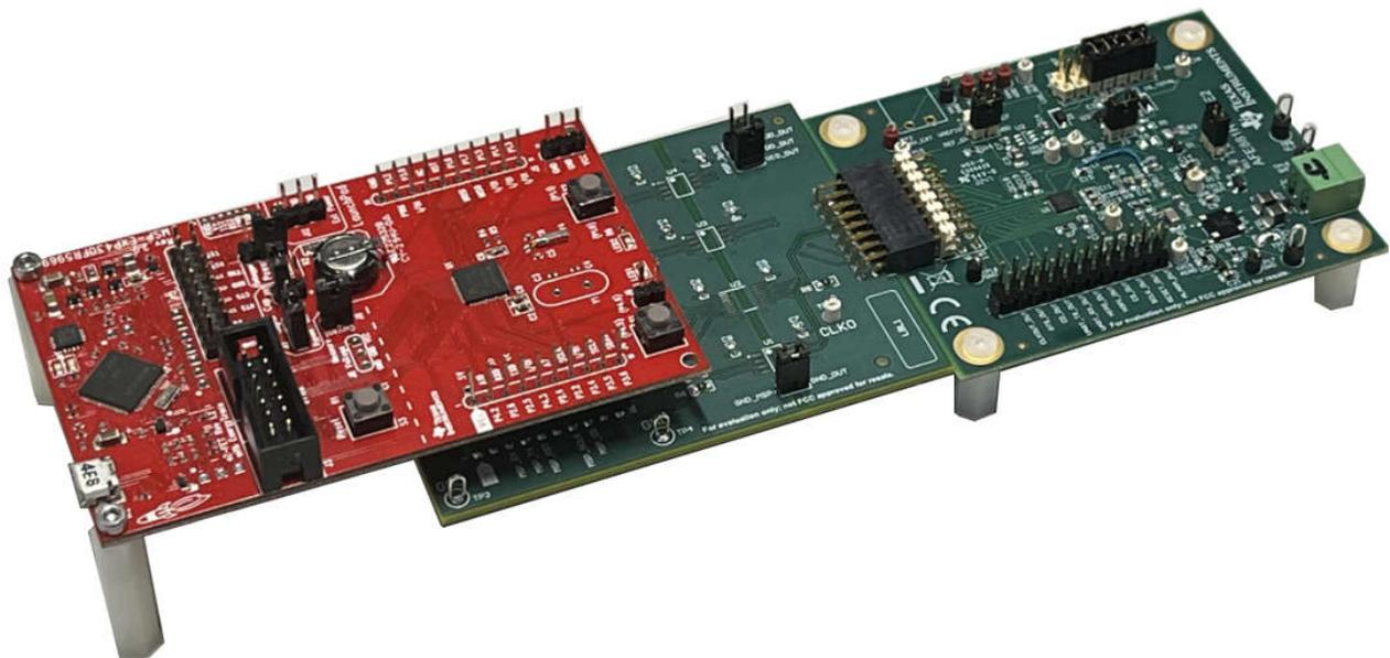
**Figure 2-12. HART Transmitter Circuit With AFE882H1-FE-EVM, DAC-LP-DBE, and MSP430 LaunchPad**
