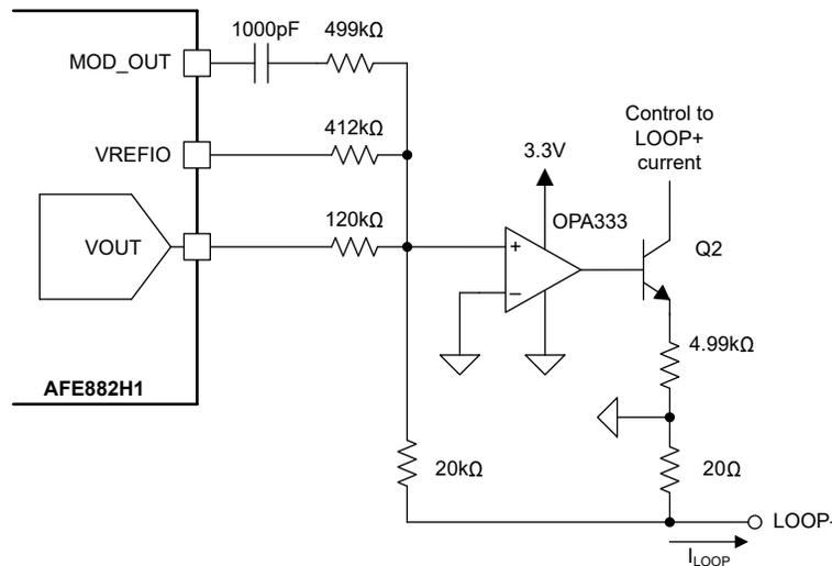
**Figure 2-10. Addition of the HART Signal From MOD\_OUT to the V-to-I Stage**
