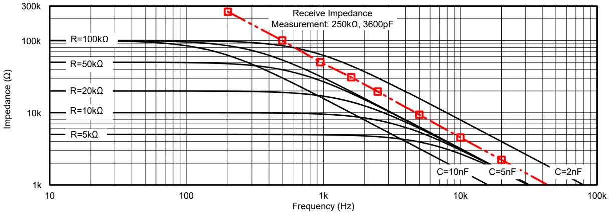
**Figure 3-18. Receive Impedance Test Results Plotted Over Frequency**
