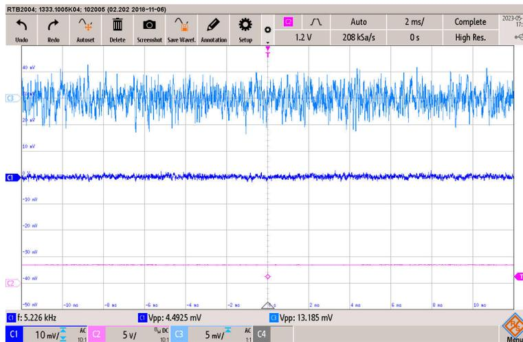
Figure 3-14. Output Noise During Silence Oscilloscope Test
