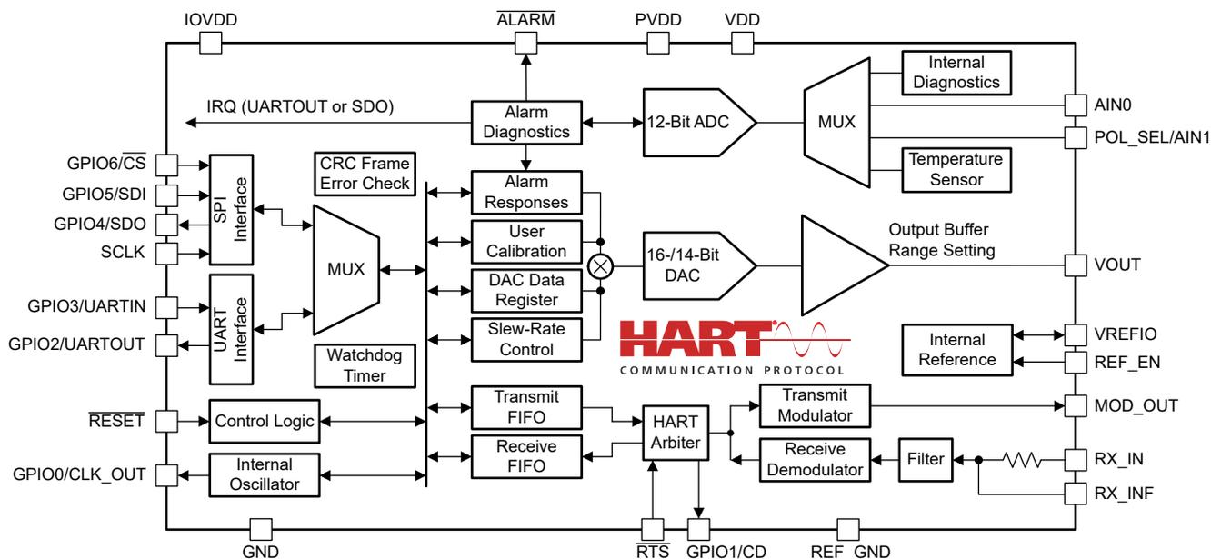
Figure 2-1. AFE882H1 Block Diagram
