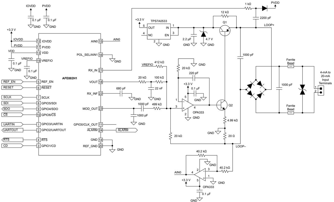
**Figure 2-6. 2-Wire Transmitter Design Using an AFE882H1 Circuit Schematic**
