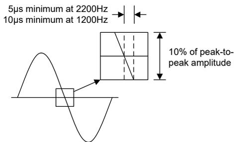
Figure 3-5. HART Sinusoidal Signaling Transition
