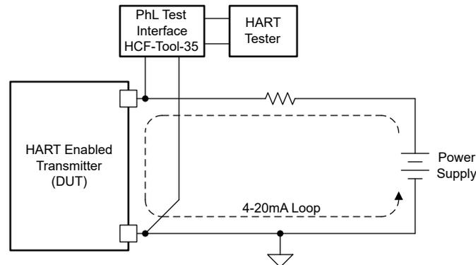
**Figure 3-20. HART Carrier Detect Test Setup**
