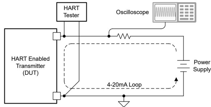
Figure 3-2. HART FSK Sinusoid Test Block Diagram
