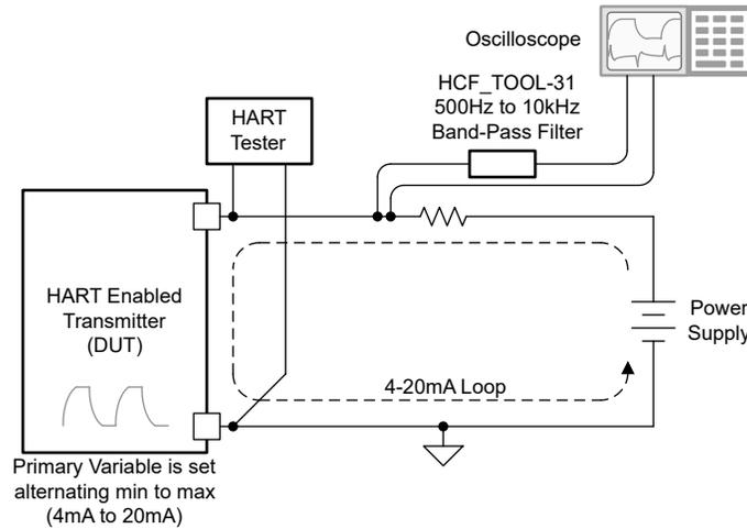
Figure 3-15. HART Analog Rate of Change Test Setup
