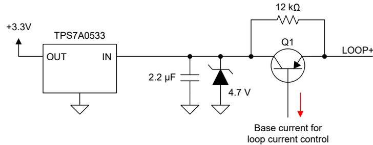
Figure 2-8. Transmitter Board Startup Circuit
