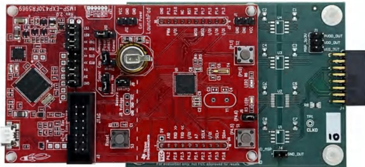
Figure 2-4. MSP-EXP430FR5969 LaunchPad with a LP-DBE Connector Board
