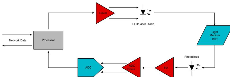
Figure 1. LiFi Signal Chain Block Diagram
