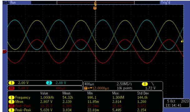
**Figure 2-10. Differential DC-Coupled Input Swing at -1dBm (0dBm = 4Vrms)**
