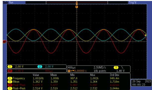
**Figure 2-2. Differential AC-Coupled Input Swing at -1dBrG (0dBrG = 2Vrms)**
