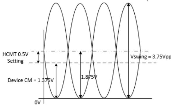
**Figure 1-2. Mode 1 Common-Mode Example**
