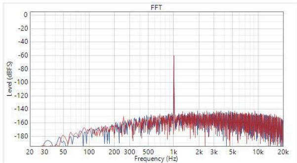
**Figure 2-3. Differential AC-Coupled Dynamic Range at -60dBrG Input**
