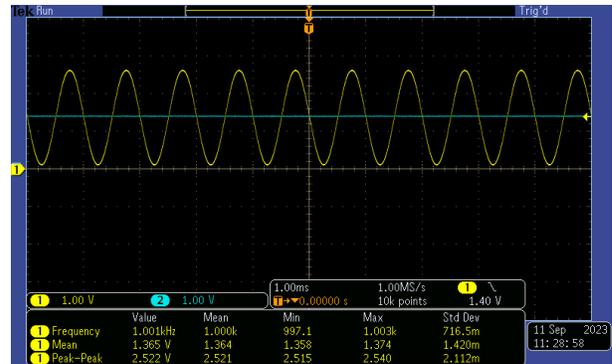
**Figure 2-6. Single Ended AC-Coupled Input Swing at -1dBrG (0dBrG = 1Vrms)**
