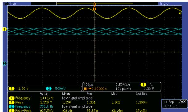
**Figure 3-6. IN1P and IN1M Input Signal**
