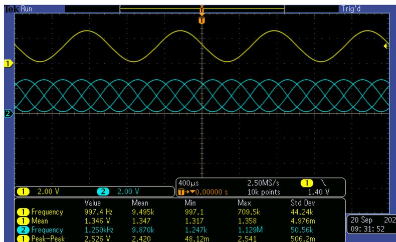
**Figure 2-19. IN1P and IN1M Mux Input at -1dBrG (0 dBrG = 1Vrms)**
