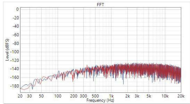
**Figure 3-4. Power Tune Mode Differential AC-Coupled SNR**
