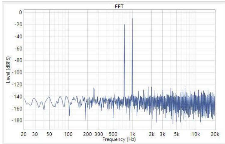
**Figure 3-7. Mixed Analog Input of IN1P and IN1M**
