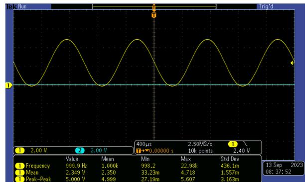
**Figure 2-14. Single Ended DC-Coupled Input Swing at -1dBrG (0dBrG = 2Vrms)**
