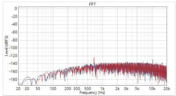
**Figure 2-8. SNR With Input AC Signal Shorted to GND**
