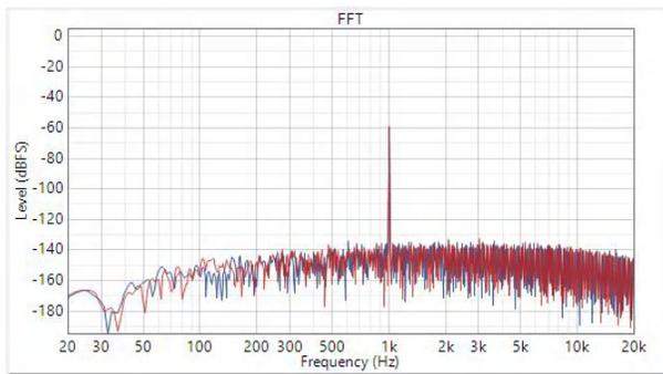
**Figure 2-15. Single Ended DC Coupling Dynamic Range with -60dBrg Input**
