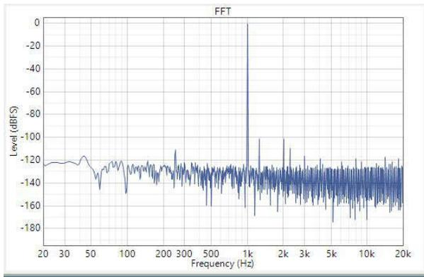
**Figure 2-20. Output with IN1P Mux Input Configured**
