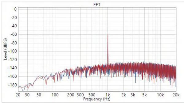
**Figure 3-3. Power Tune Mode Differential AC-Coupled Dynamic Range at -60dBrg**
