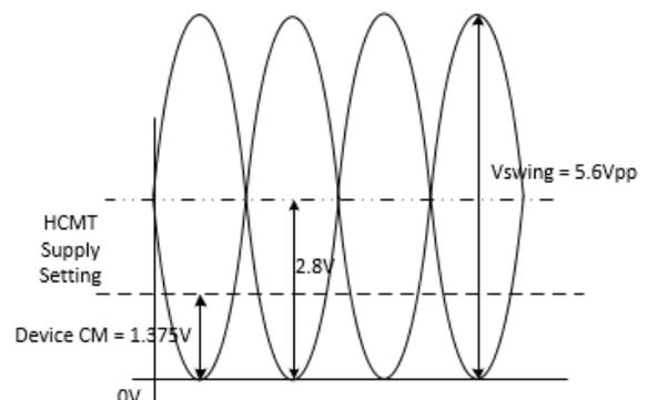
**Figure 1-3. Mode 2 Common-Mode Example**
