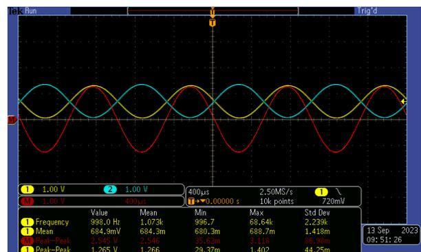
**Figure 3-2. Power Tune Differential AC-Coupled Input at -1dBrG (0dBrG = 1Vrms)**
