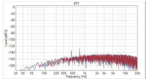
**Figure 2-4. SNR with Input AC Signal shorted to GND**
