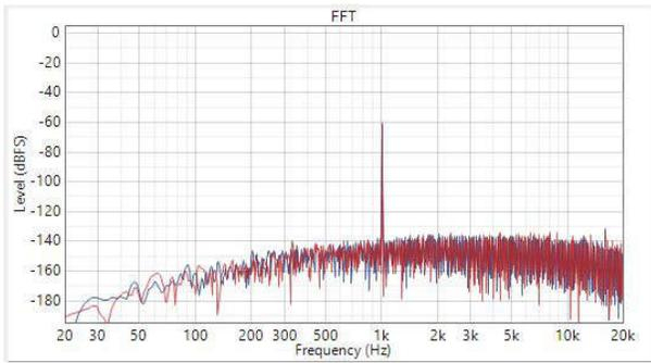
**Figure 2-7. Single Ended AC-Coupled Dynamic Range at -60dBm Input**
