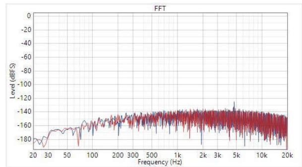
**Figure 2-16. Single Ended DC Coupling SNR**
