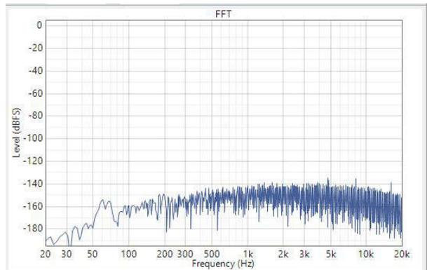
**Figure 2-12. SNR with Input AC Signal shorted to GND**
