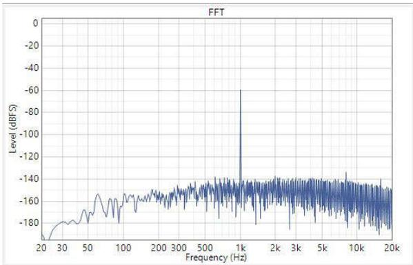
**Figure 2-11. Differential DC-Coupled Dynamic Range at -60dBm Input**
