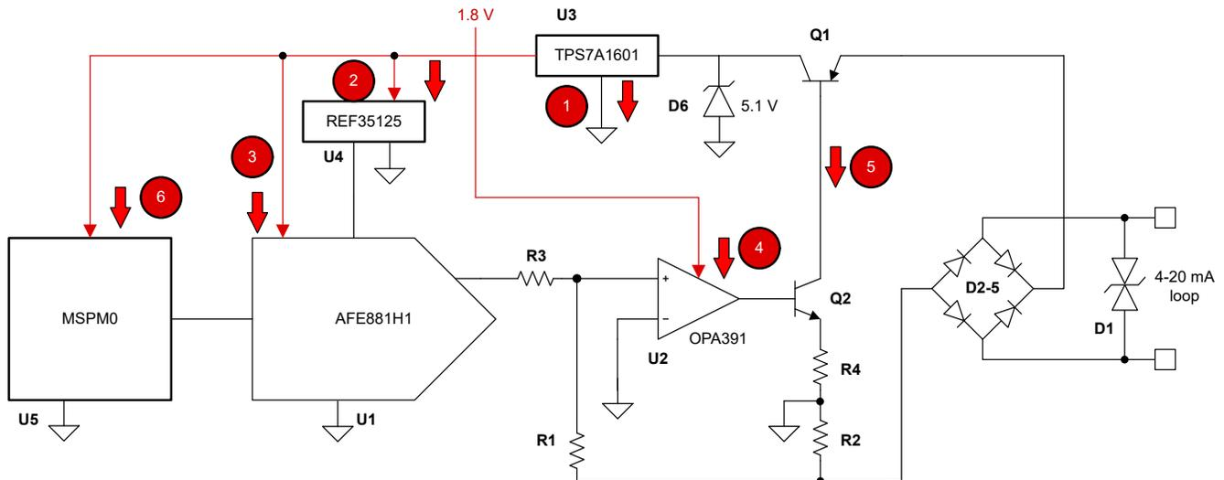
**Figure 3. Different Current Components of the Transmitter Circuit**
