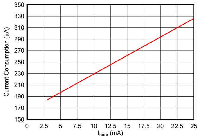
**Figure 4. Total Current Consumption vs Loop Current**
