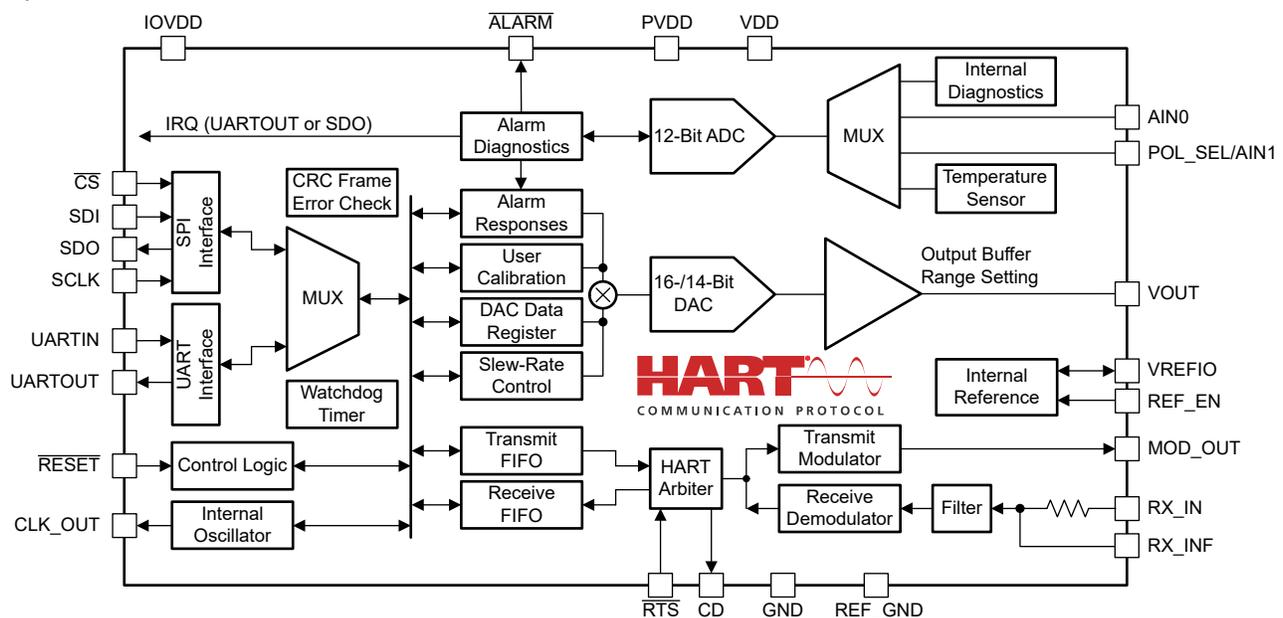
Figure 1. AFE881H1 Block Diagram
