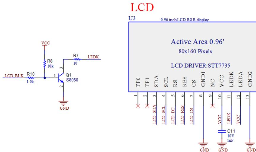
Figure 3-4. Schematic Diagram of LCD
