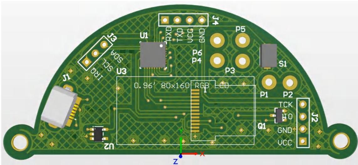
Figure 3-5. PCB and Circuit Board of Liquid Level Measurement Application
