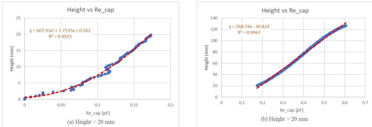
Figure 3-14. Height vs Relative Capacitance Change Curve Fit (Software Optimization)
