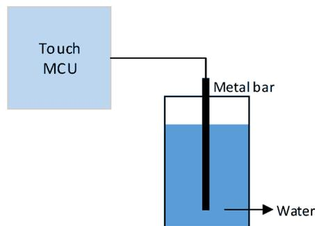
Figure 1-1. Simplified Schematic of Liquid Level Detection System
