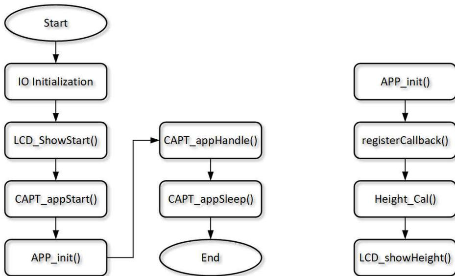
**Figure 3-7. Overall Code Design Flow Chart**
