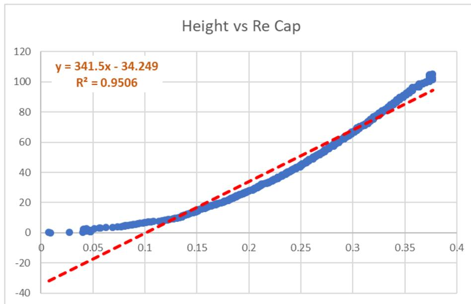
Figure 3-6. Correspondence Between Height and Capacitance Change
