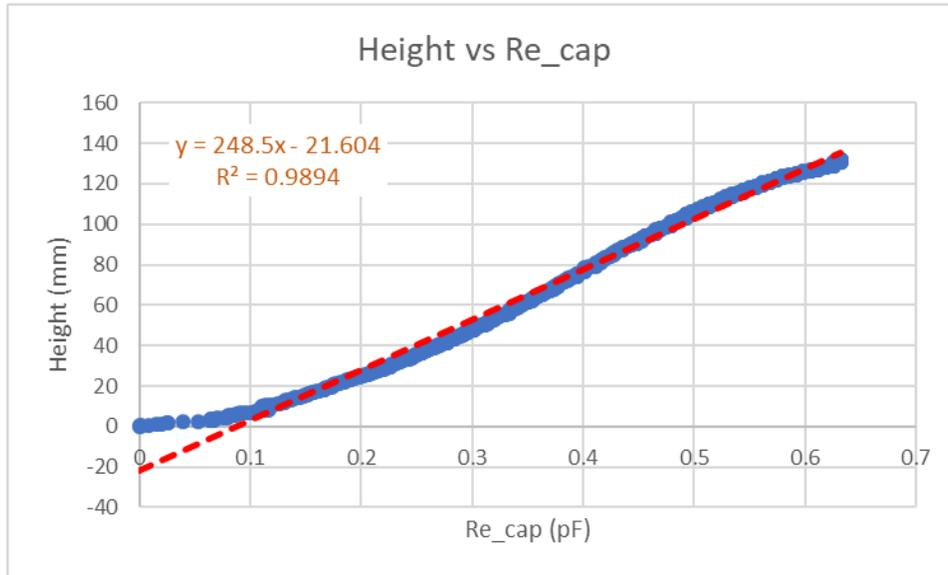
Figure 3-13. Height vs Relative Capacitance Change Curve Fit
