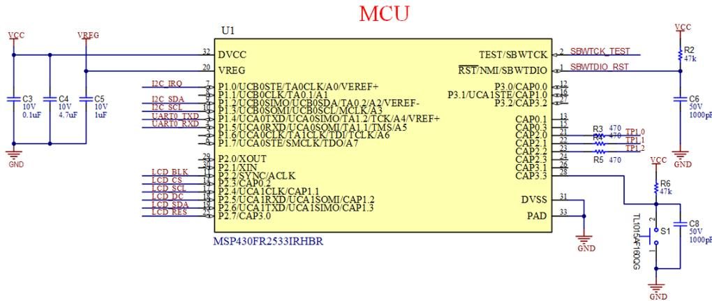
Figure 3-3. Schematic Diagram of MSP430FR2533
