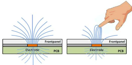
**Figure 2-1. Self-Capacitive Detection**
