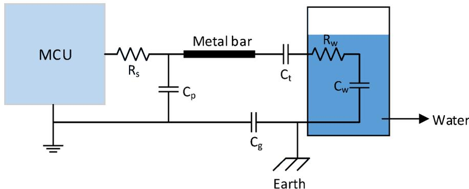
**Figure 2-3. Liquid Level Detection Model**
