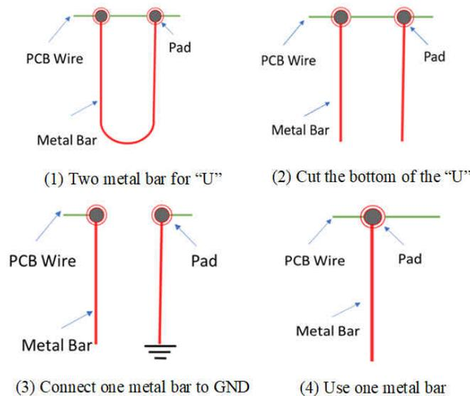
Figure 3-9. Four Different Electrode Connection Tests
