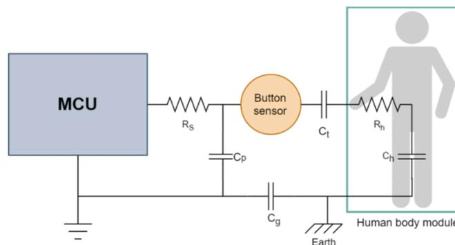
**Figure 2-2. Self-Capacitive Detection Model**
