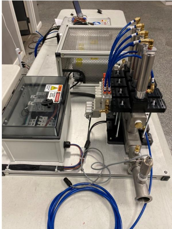
**Figure 3-1. Sonic Nozzle Test and Calibration System**
