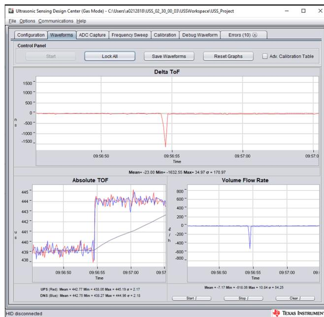
Figure 3-2. Level-Sensing Test Results
