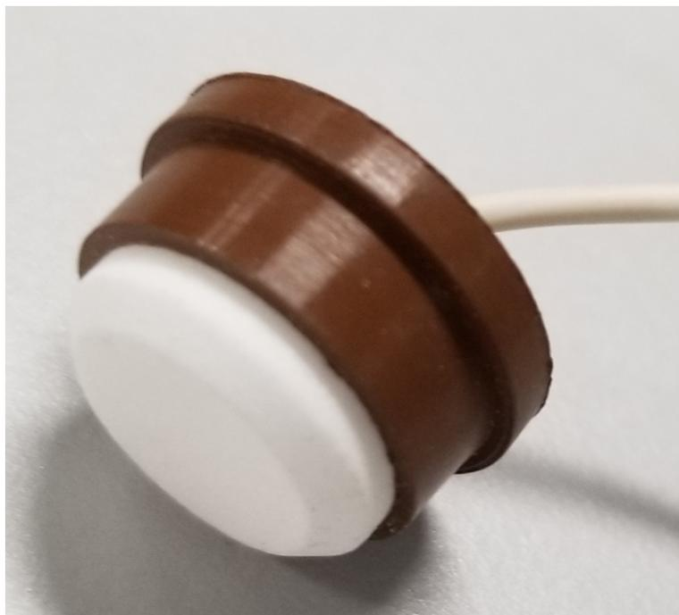
**Figure 2-2. Jiakang 200-kHz Transducer**
