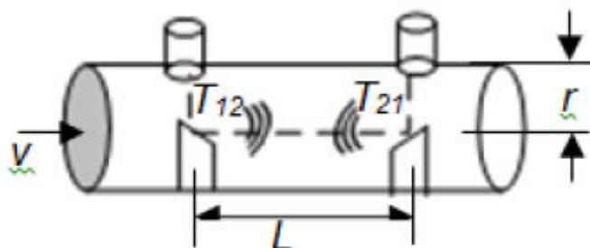
**Figure 2-1. Typical Ultrasonic Water Meter**
