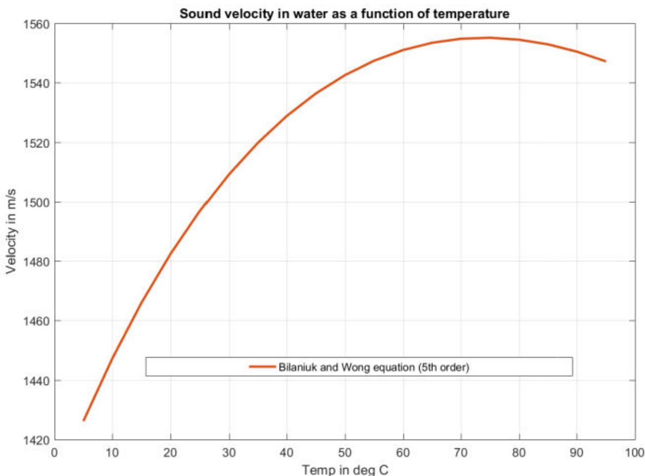
**Figure 2-4. Temperature vs. Sound velocity in water**
