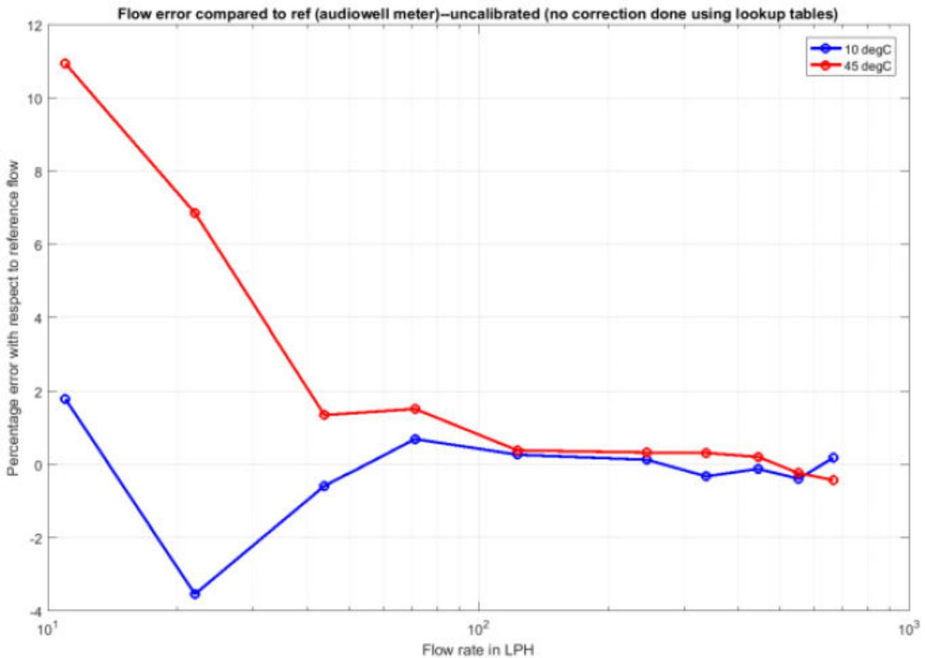
**Figure 2-3. Flow Error Curves for 10°C and 45°C DN20 Meter**
