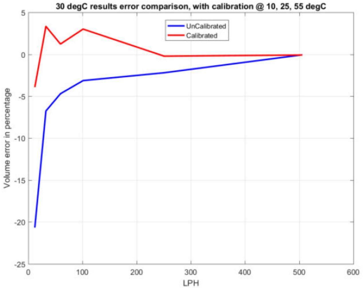
Figure 4-2. Calibrated and Uncalibrated Volume Flow Error at 30°C
