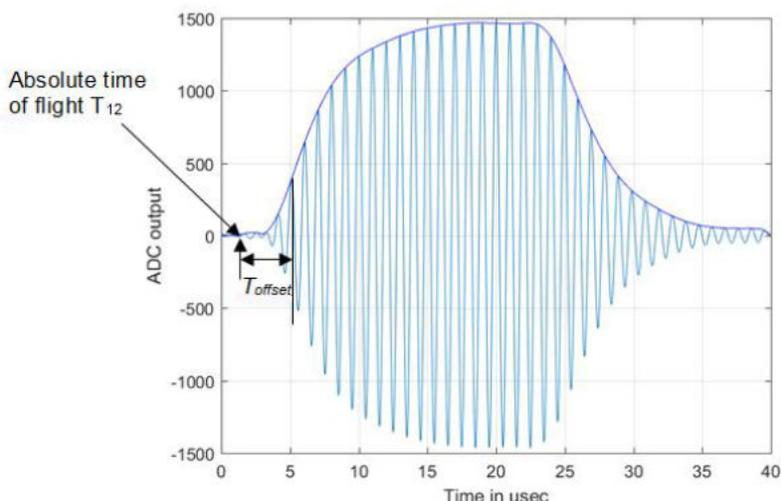
**Figure 2-2. Typical Waveform Arrival and Definition of Absolute Time of Flight**
