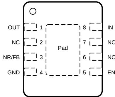
**Figure 4-2. Pin Diagram (VSON (DRB) Package)**
