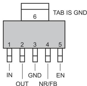
**Figure 4-1. Pin Diagram (SOT-223 (DCQ)) Package**
