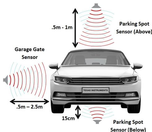
Figure 2. Mounting for Vehicle Detection
