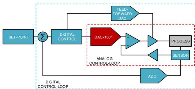
Figure 1. Feedback Control Loop
