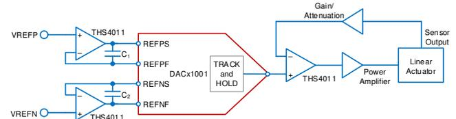
Figure 2. DACx1001 Control Loop Schematic
