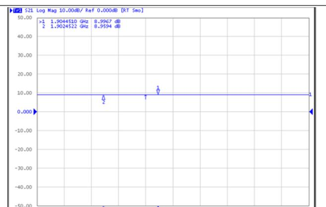
Figure 14. Gain Measurement: Gain is Flat at 9 dBm With TX/RX DSA Set to 0
