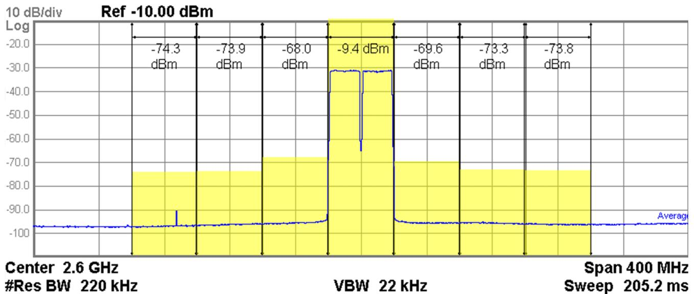
Figure 15. TX Output : 2x20MHz LTE Signal at 2.6GHz
