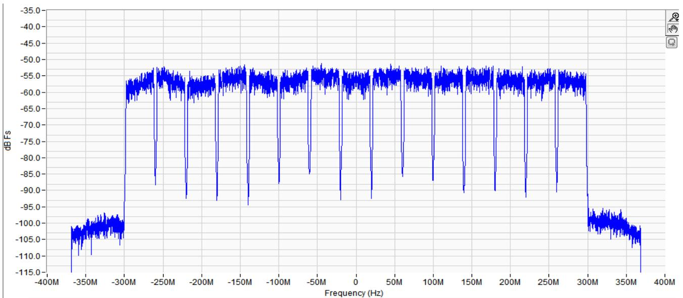
Figure 19. FBRX Path Output with Wideband Signal (600MHz)
