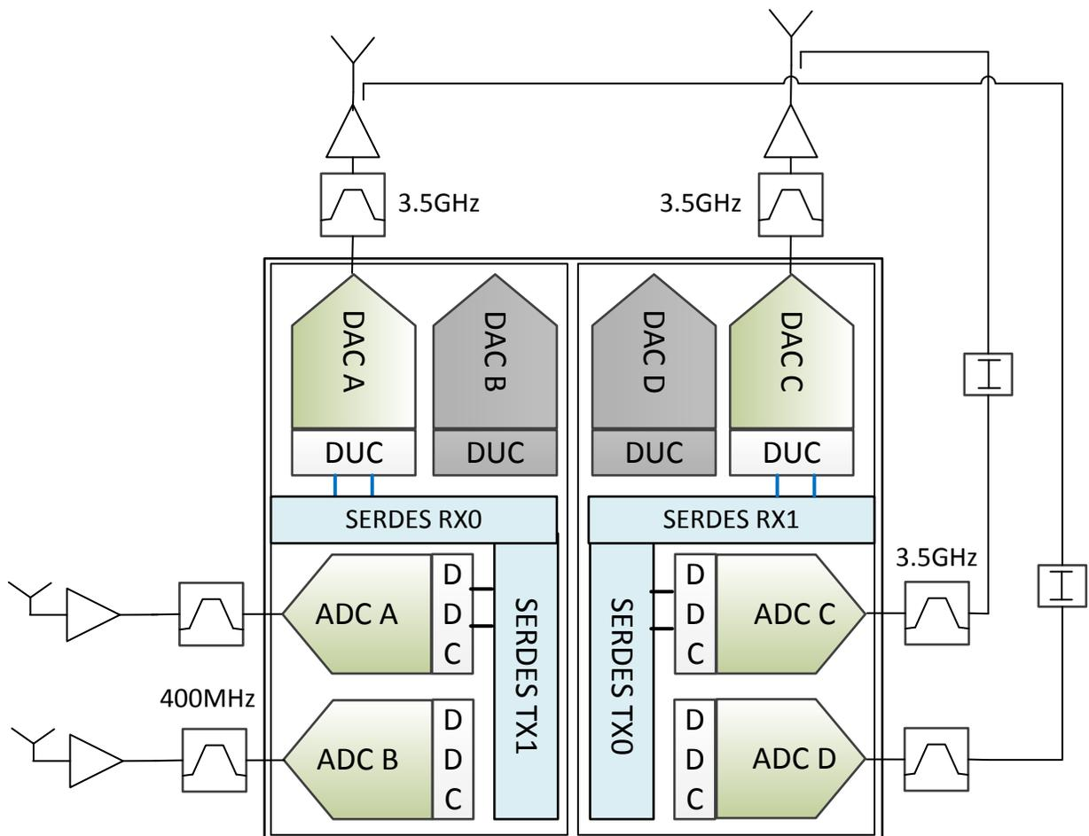
**Figure 12. 2T2R2FB Configuration for RF Repeater**
