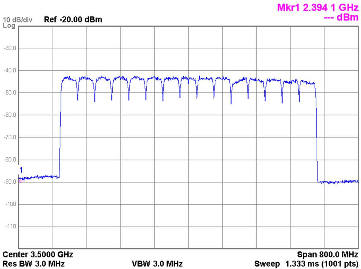
Figure 18. TX Path Output with Wideband Signal (600MHz)
