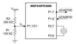
Figure 1. Voltage Monitor Block Diagram
