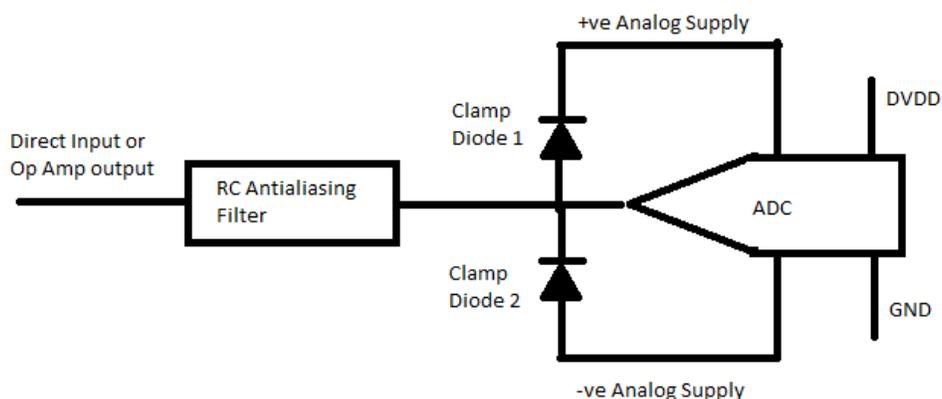
Figure 2. Input Protection Using Clamps
