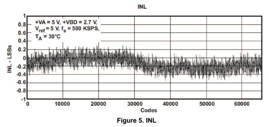
INL value is usually specified using one of the following units: LSB or %FSR.
