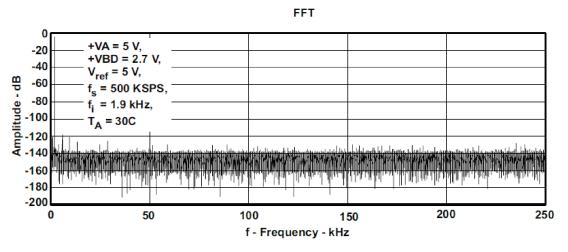
Figure 6. Typical ADC Output Spectrum Plot
