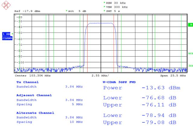
Figure 19. 103.304-MHz DAC Output Under Spurious Free Clock
