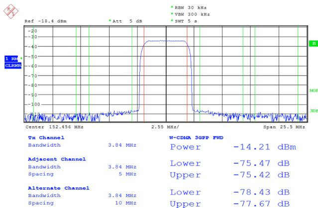
Figure 23. 152.456-MHz DAC Output Under Spurious Free Clock
