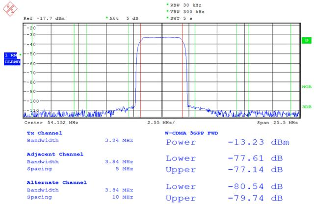
Figure 15. 54.152-MHz DAC Output Under Spurious Free Clock
