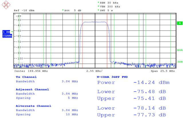
Figure 21. 149.956-MHz DAC Output Under Spurious Free Clock
