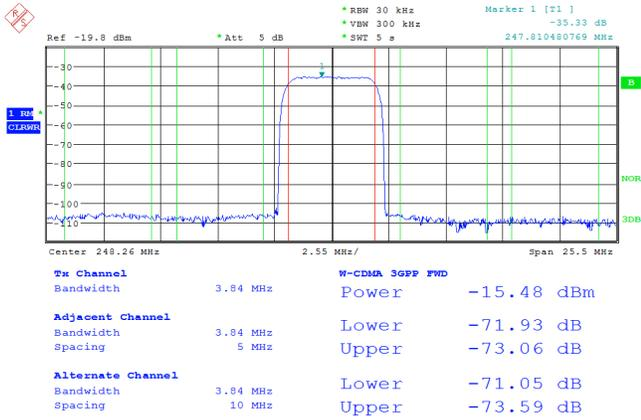
Figure 25. 248.26-MHz DAC Output Under Spurious Free Clock
