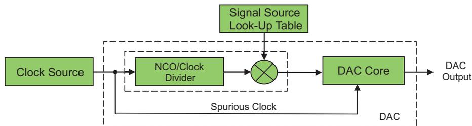
**Figure 4. Signal Flow Diagram of DAC3482**
