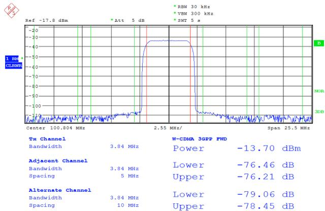
Figure 17. 100.804-MHz DAC Output Under Spurious Free Clock
