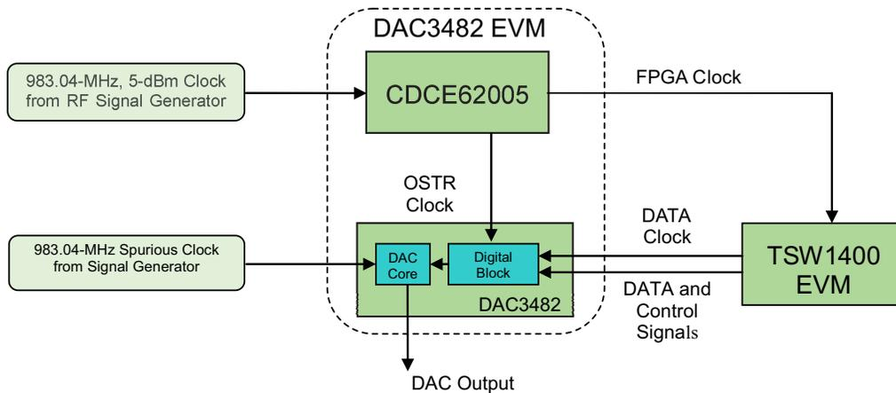
Figure 1. EVM Setup for Test
