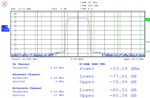
Figure 13. 51.652-MHz DAC Output Under Spurious Free Clock
