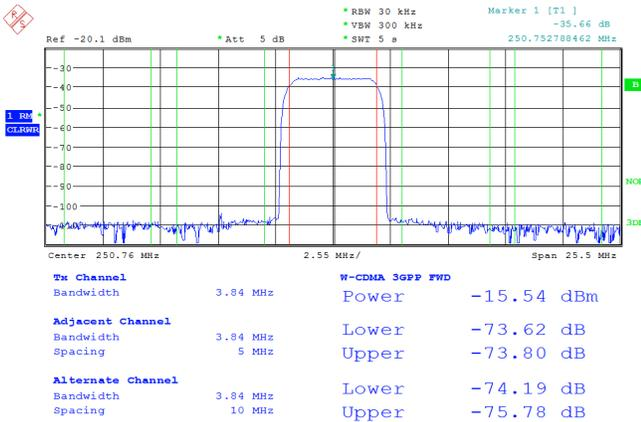
Figure 27. 250.76-MHz DAC Output Under Spurious Free Clock
