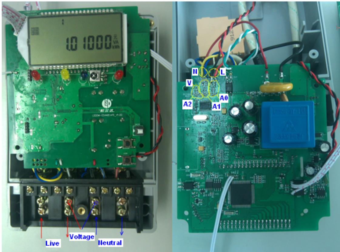
Figure 12. Demo E-Meter Connection for CSG Test
