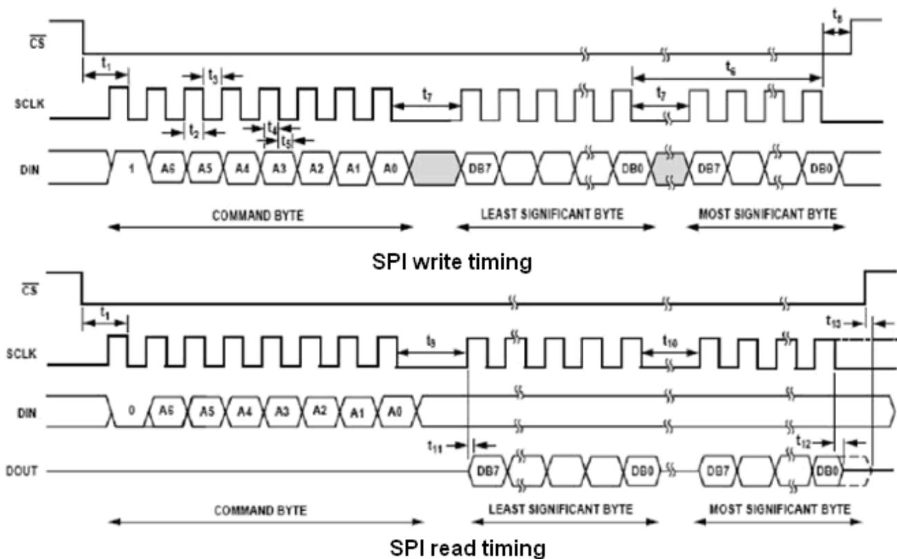
Figure 17. SPI Timing
