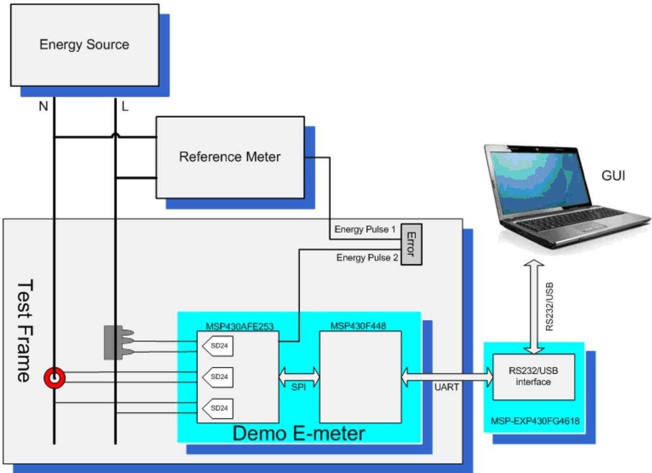
Figure 2. Test System Setup
