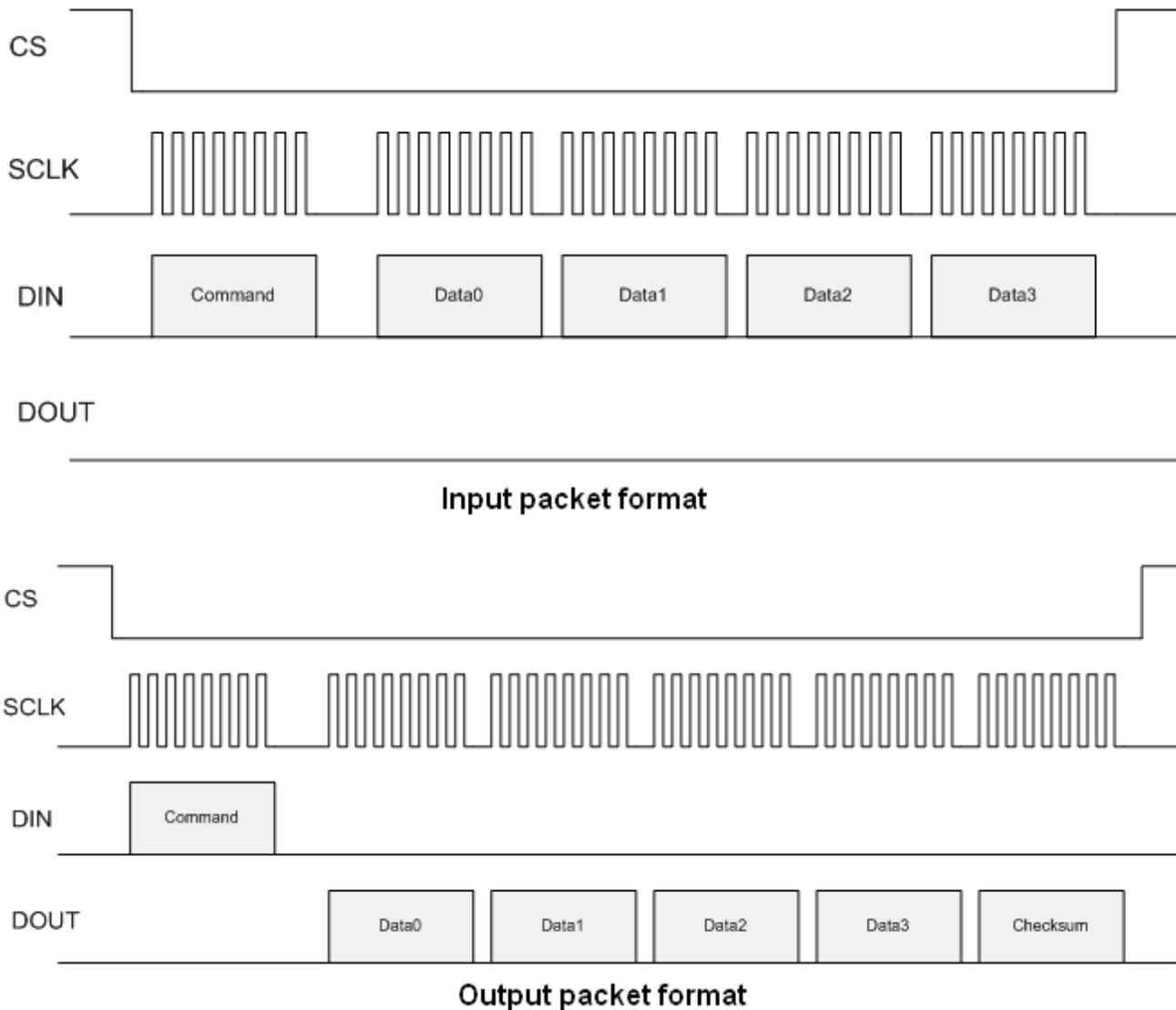
**Figure 18. CSG Firmware Communication Packet**
