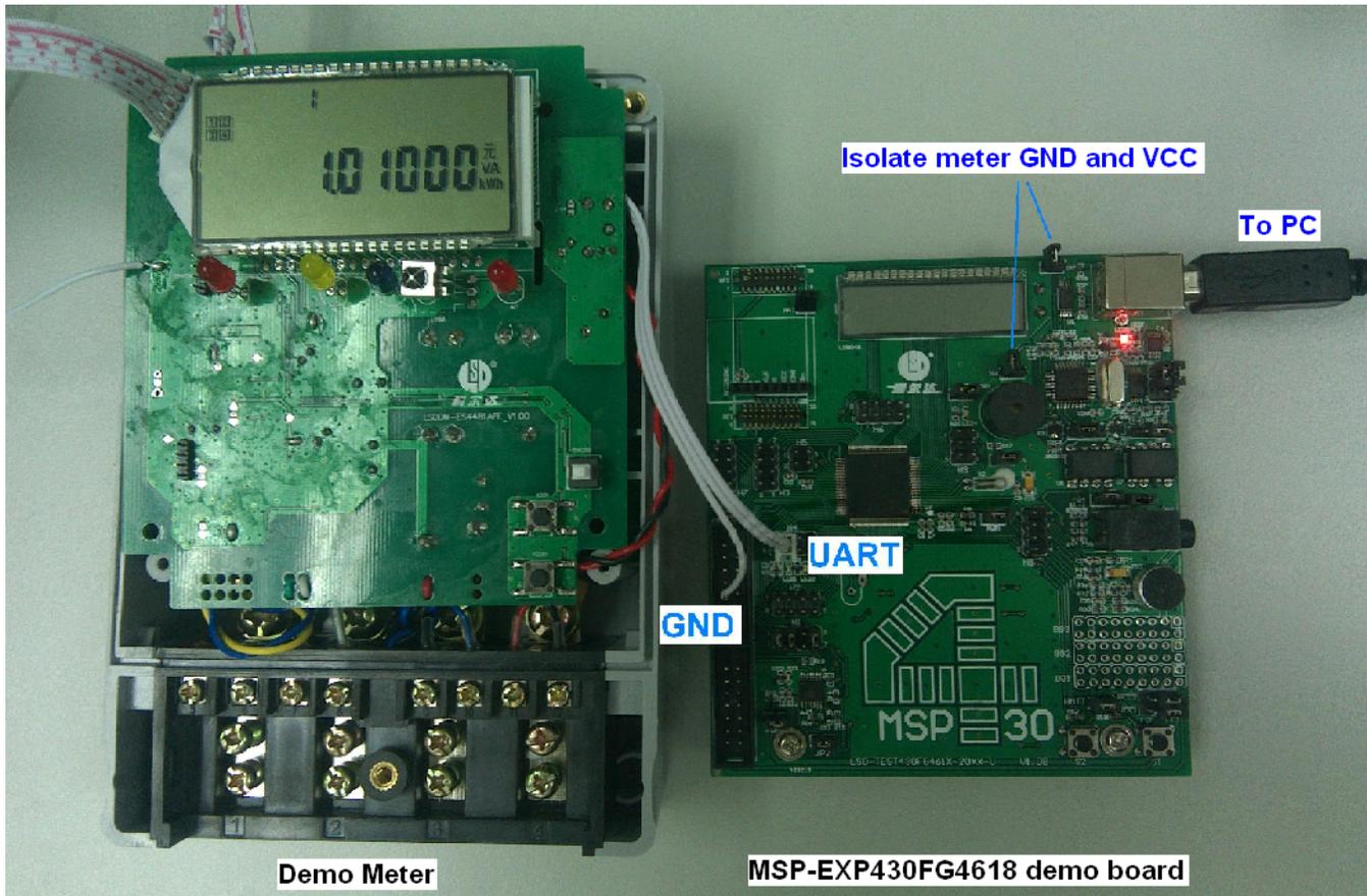
Figure 3. Connection Between Demo Meter and MSP-EXP430FG4618 Demo Board
