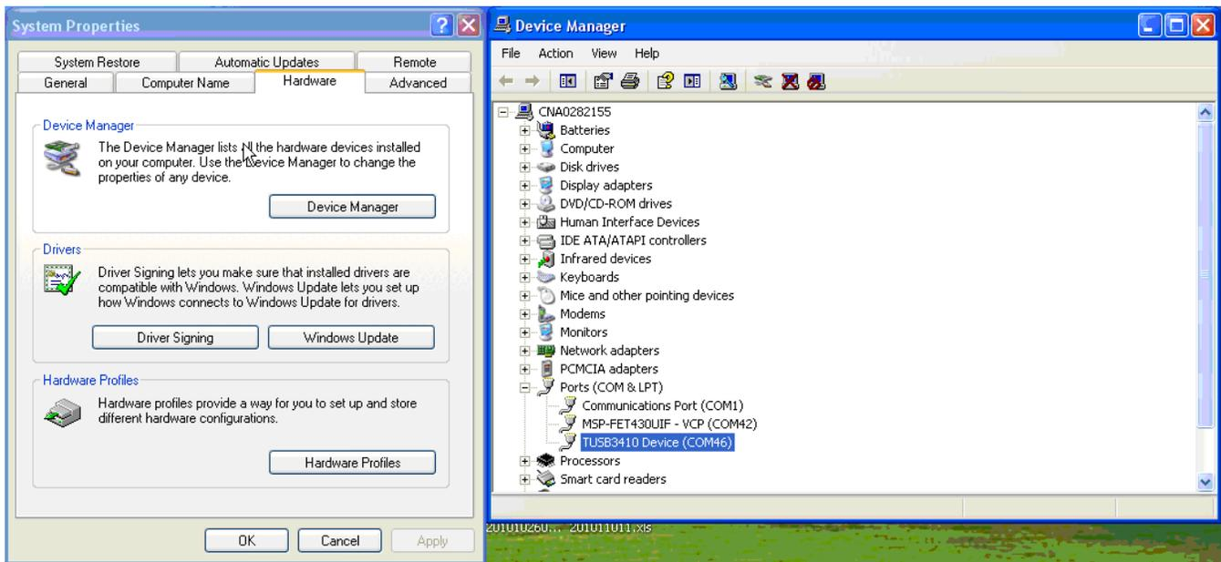
Figure 4. Check Serial Port Number for MSP-EXP430FG4618 Demo Board
