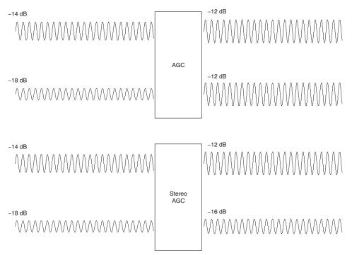
Figure 1. Stereo AGC Operation
