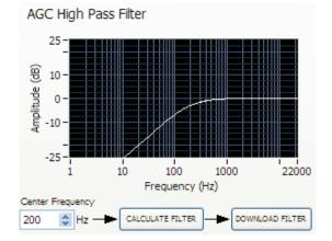
Figure 10. AGC High-Pass Filter
