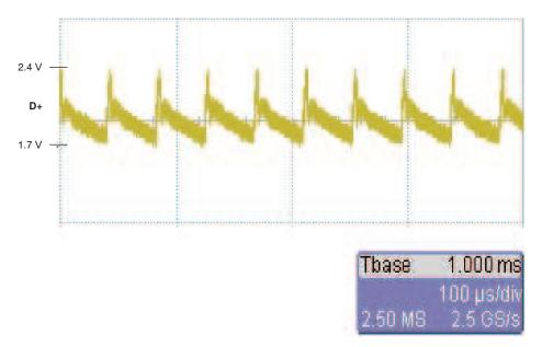
Figure 3. Oscillations on D+ Line as a Result of an Unstable V<sub>DDi</sub> (Enlarged)
