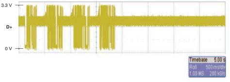
Figure 2. Oscillations on D+ Line as a Result of an Unstable V<sub>DDi</sub>
