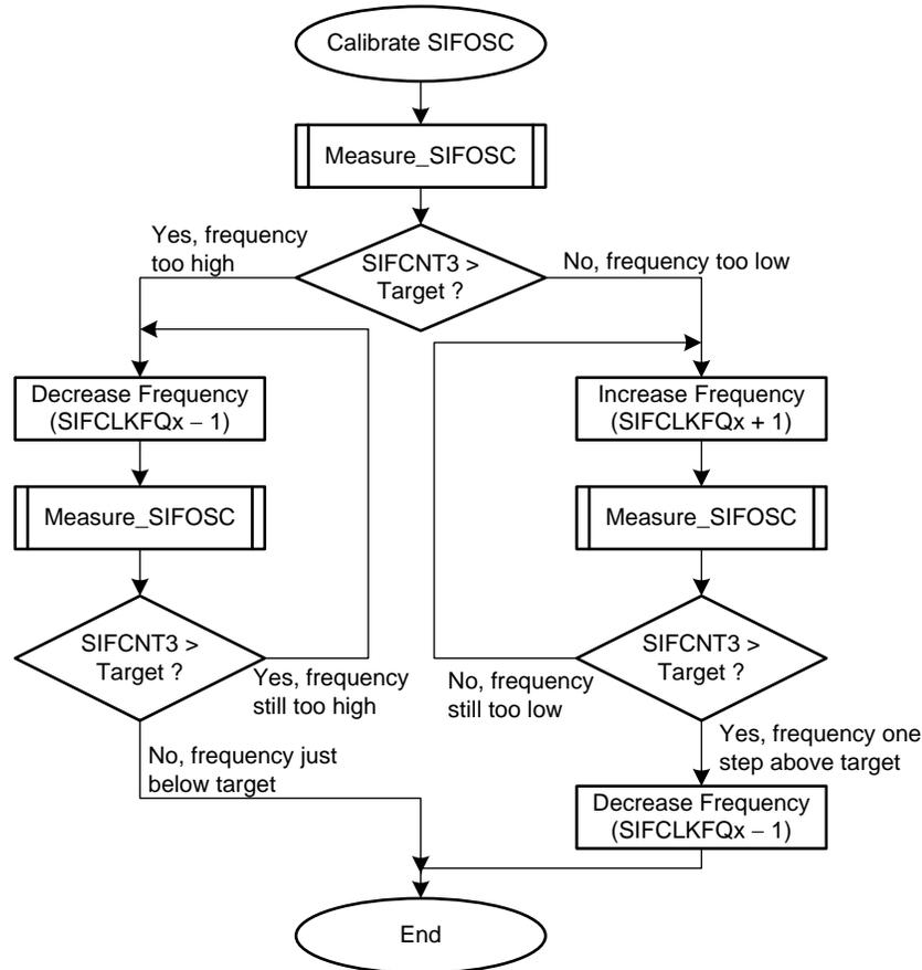
Figure 3. Algorithm to Calibrate Scan Interface Oscillator SIFOSC
