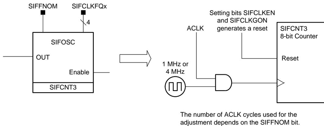
**Figure 1. Scan Interface Timing State Machine Oscillator (SIFOSC)**
