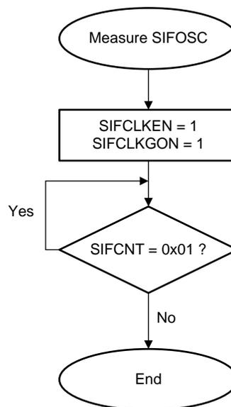
**Figure 2. Algorithm to Measure Scan Interface Internal Oscillator**
