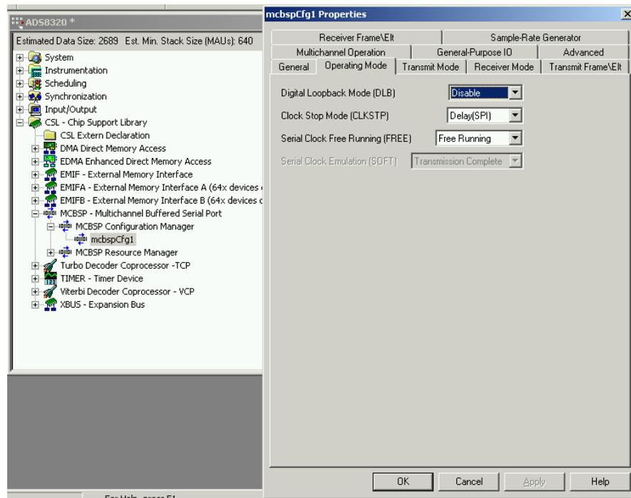
Figure 2. Operating Mode Tab
