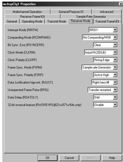
**Figure 5. Receive Mode Tab**
