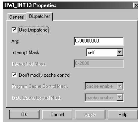
Figure 10. McBSP1Rcv\_ISR Dispatcher Tab
