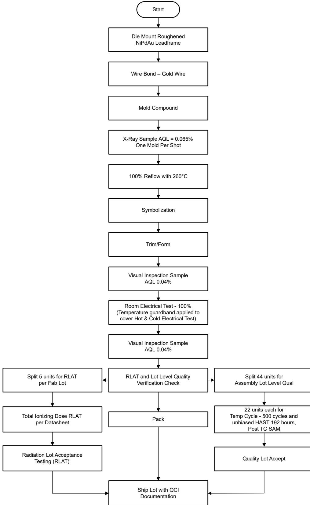
Figure 1-1. SN54SC1G175-SEP Space Enhanced Plastic Production Flow Chart
